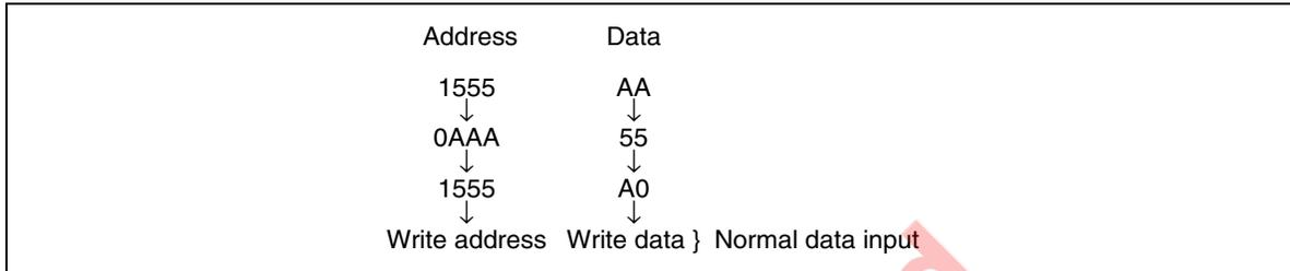
Software data protection mode can be canceled by inputting the following 6 bytes. After that, this device turns to the non-protection mode and can write data normally. But when the data is input in the canceling cycle, the data cannot be written.
