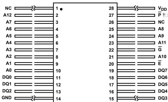
†  $\bar{P}$  must be hardwired at all times to  $V_{DD}$ , except during programming.
