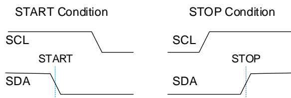
Figure 14. START and STOP Condition Waveform
