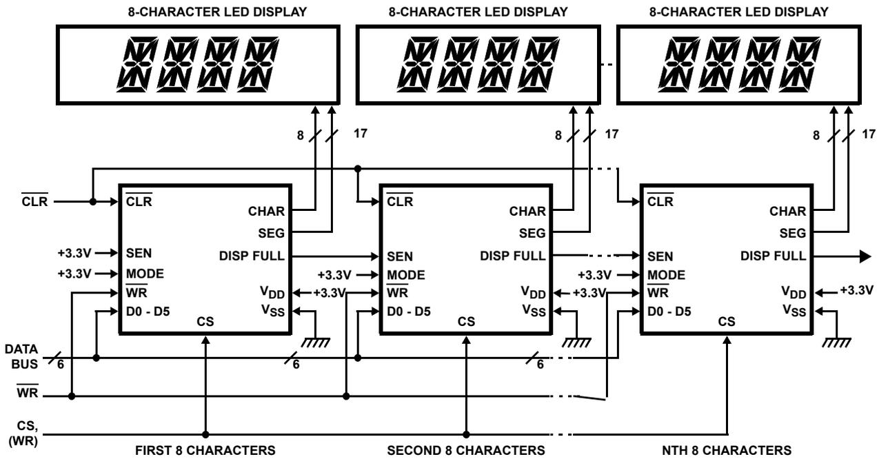
FIGURE 6. MULTICHARACTER DISPLAY USING SEQUENTIAL ACCESS MODE
