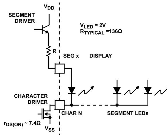
FIGURE 10. SEGMENT AND CHARACTER DRIVERS OUTPUT CIRCUIT
