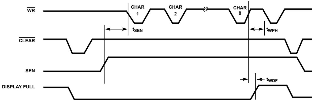
FIGURE 2. SEQUENTIAL ACCESS MODE TIMING (MODE = 1)
