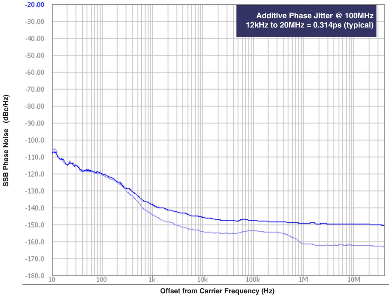
As with most timing specifications, phase noise measurements has issues relating to the limitations of the equipment. Often the noise floor of the equipment is higher than the noise floor of the device. This is illustrated above. The device meets the noise floor of what is shown, but can actually be lower. The phase noise is dependent on the input source and measurement equipment.
