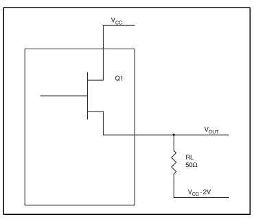
Figure 6. LVPECL Driver Circuit and Termination
