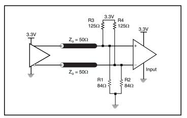
Figure 4B. 3.3V LVPECL Output Termination
