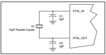
Figure 2A. Crystal Input Interface, using 12pF crystal
