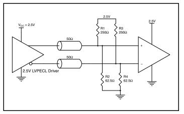
Figure 5A. 2.5V LVPECL Driver Termination Example
