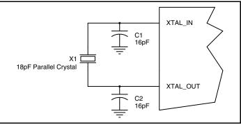
Figure 2B. Crystal Input Interface, using 18pF crystal
