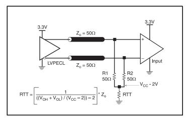
Figure 4A. 3.3V LVPECL Output Termination
