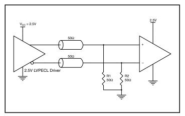
Figure 5C. 2.5V LVPECL Driver Termination Example
