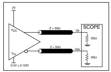
2.5V LVPECL Output Load AC Test Circuit
