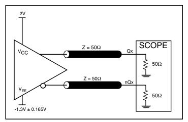
3.3V LVPECL Output Load AC Test Circuit
