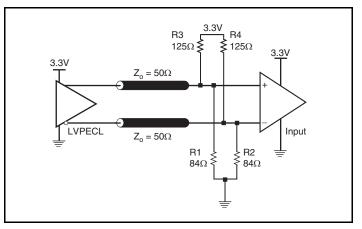
Figure 2B. 3.3V LVPECL Output Termination
