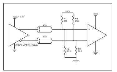
Figure 3A. 2.5V LVPECL Driver Termination Example
