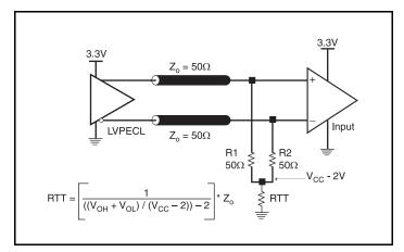
Figure 2A. 3.3V LVPECL Output Termination
