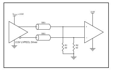
Figure 3C. 2.5V LVPECL Driver Termination Example
