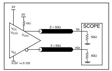
2.5V LVPECL Output Load AC Test Circuit
