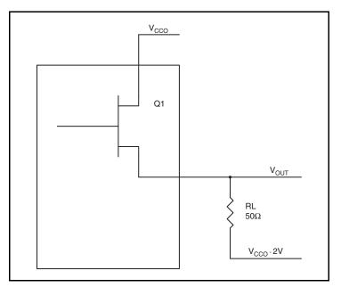
Figure 6. LVPECL Driver Circuit and Termination
