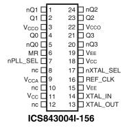
24-Lead TSSOP, E-Pad 4.4mm x 7.8mm x 0.925mm package body G Package Top View
