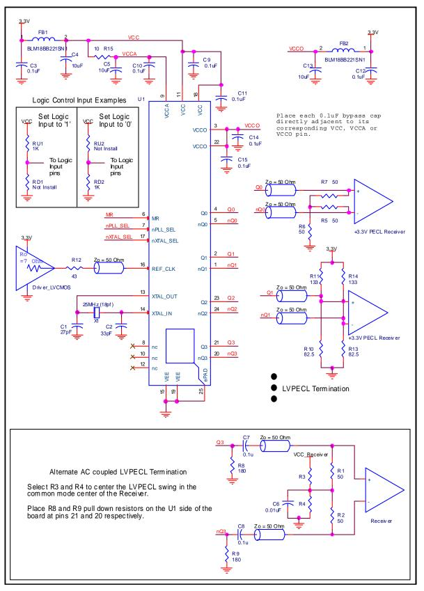
Figure 5. ICS843004I-156 Application Schematic
