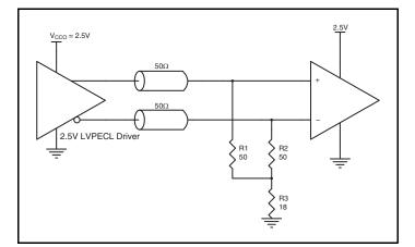
Figure 3B. 2.5V LVPECL Driver Termination Example
