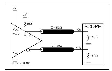
3.3V LVPECL Output Load AC Test Circuit
