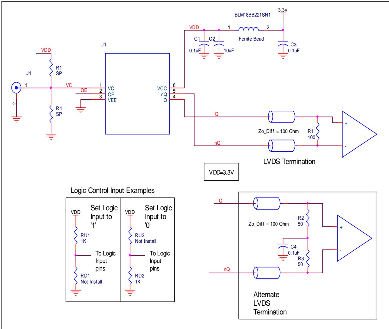
Figure 2. IDT8N4SV75 Schematic Example
