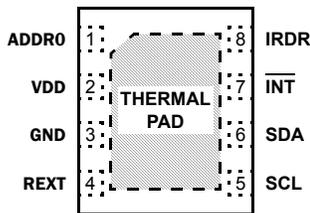
\*THERMAL PAD CAN BE CONNECTED TO GND OR ELECTRICALLY ISOLATED
