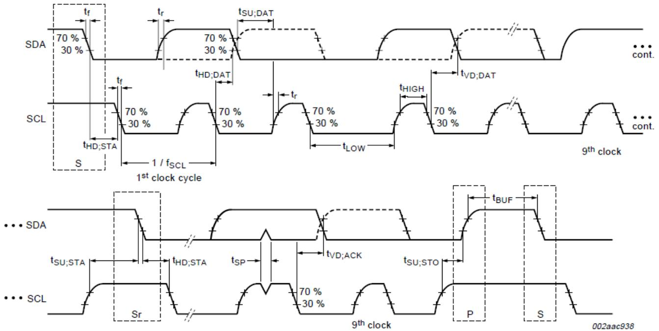
FIGURE 1. I<sup>2</sup>C TIMING DIAGRAM
