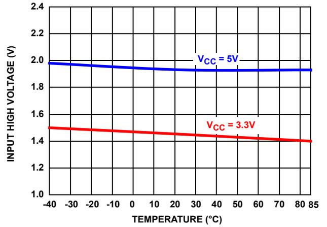
FIGURE 33. LOGIC INPUT HIGH VOLTAGE vs TEMPERATURE
