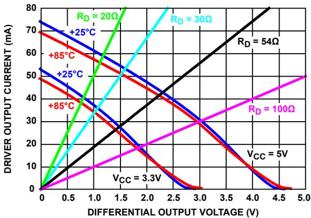
FIGURE 12. DRIVER OUTPUT CURRENT vs DIFFERENTIAL OUTPUT VOLTAGE
