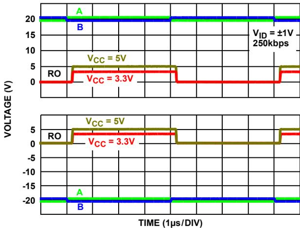
FIGURE 24.  $\pm 20\text{V}$  RECEIVER PERFORMANCE (ISL32450E, ISL32452E, ISL32457E)
