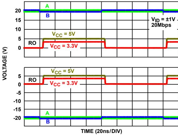
FIGURE 26.  $\pm 20\text{V}$  RECEIVER PERFORMANCE (ISL32458E, ISL32459E)
