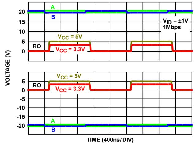
FIGURE 25.  $\pm 20\text{V}$  RECEIVER PERFORMANCE (ISL32453E, ISL32455E)
