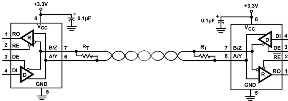
FIGURE 4. ISL32452E, ISL32455E, ISL32458E HALF DUPLEX NETWORK
