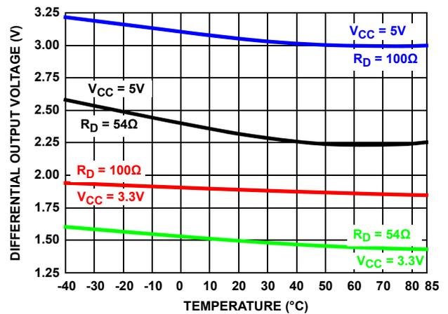
FIGURE 13. DRIVER DIFFERENTIAL OUTPUT VOLTAGE vs TEMPERATURE
