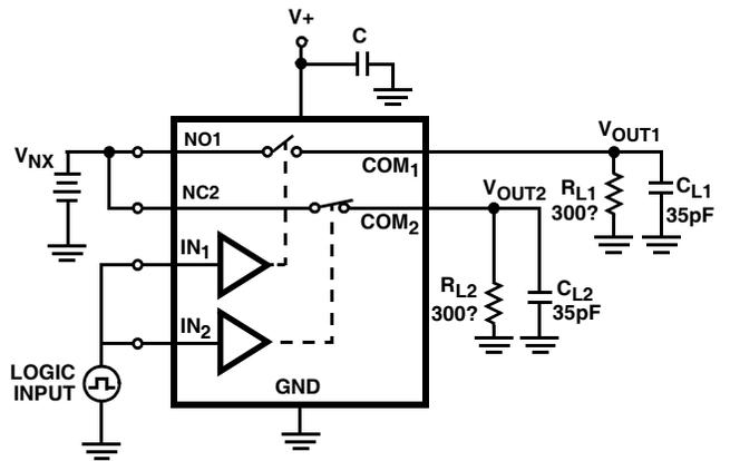
$C_L$  includes fixture and stray capacitance.
