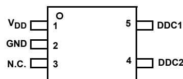
ISL54103 (5 LD SOT-23) TOP VIEW
