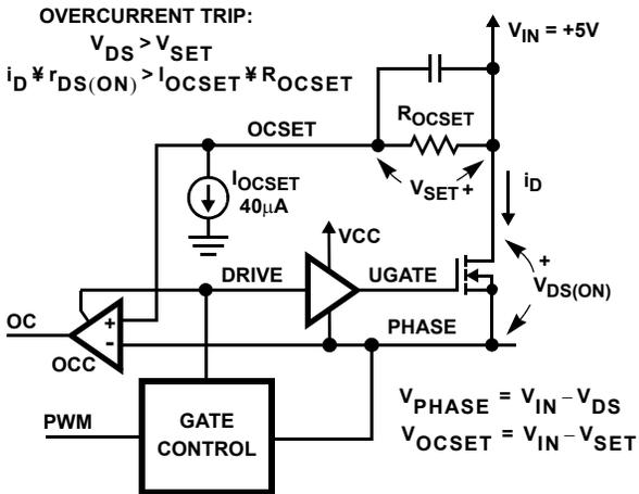
FIGURE 3. OVERCURRENT DETECTION
