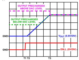
FIGURE 7. SOFT-START WAVEFORMS FOR ISL6563-BASED MULTIPHASE CONVERTER
