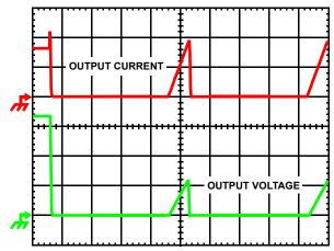
FIGURE 4. OVERCURRENT BEHAVIOR IN HICCUP MODE
