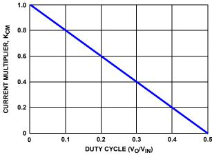
FIGURE 10. RIPPLE CURRENT vs DUTY CYCLE
