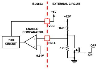
FIGURE 6. START-UP COORDINATION USING THRESHOLD-SENSITIVE ENABLE (ENLL) PIN
