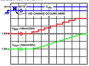
FIGURE 5. TYPICAL DYNAMIC-VID OPERATION, VRM9 DAC SETTING
