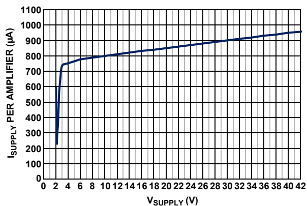
FIGURE 26. SUPPLY CURRENT vs SUPPLY VOLTAGE
