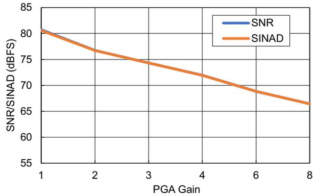
Figure 71. SNR and SINAD vs PGA Gain
