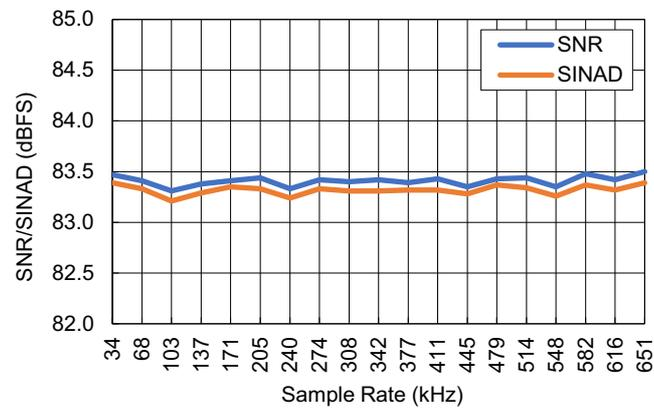
Figure 77. SNR and SINAD vs Sample Rate
