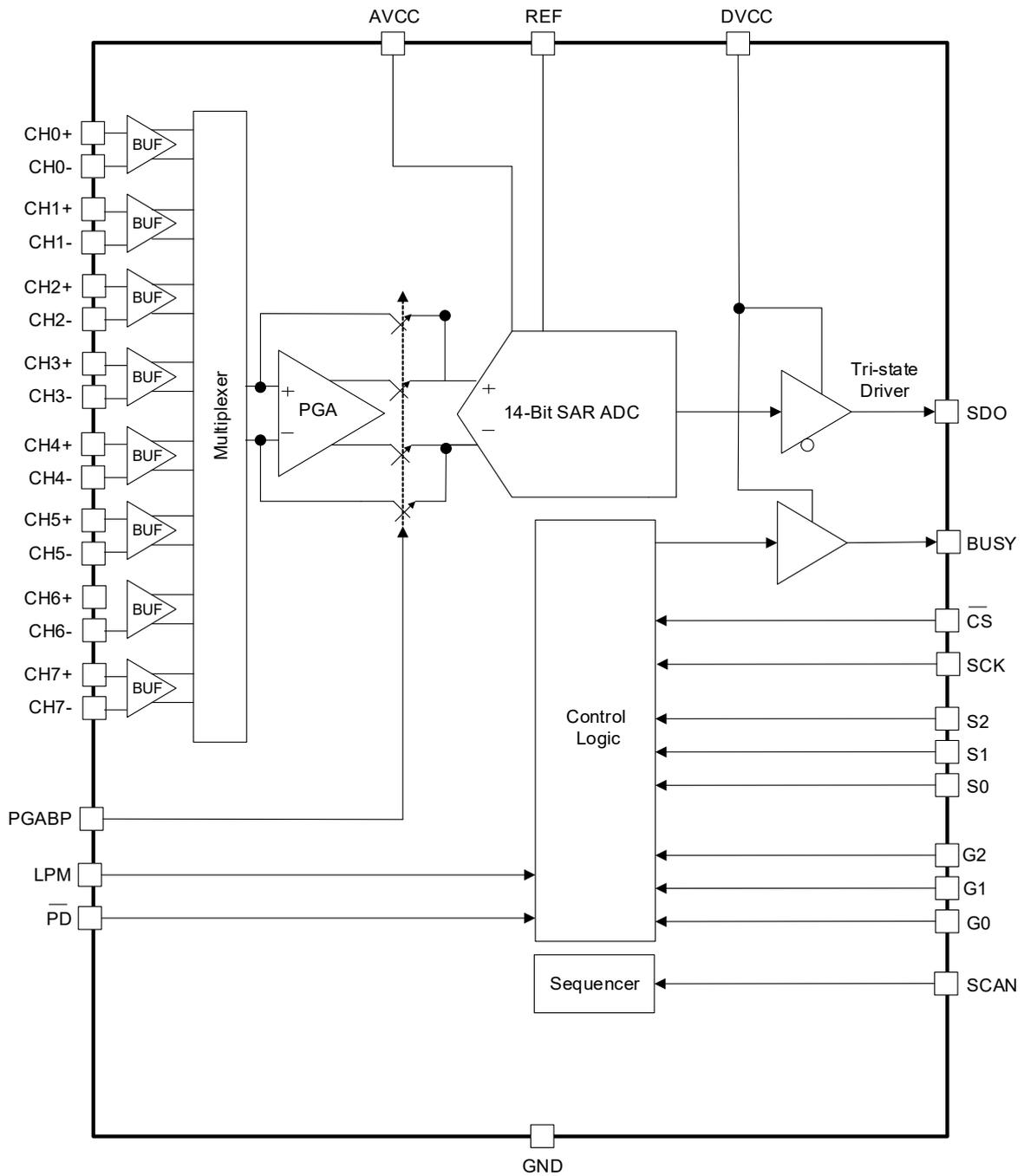
Figure 4. Block Diagram
