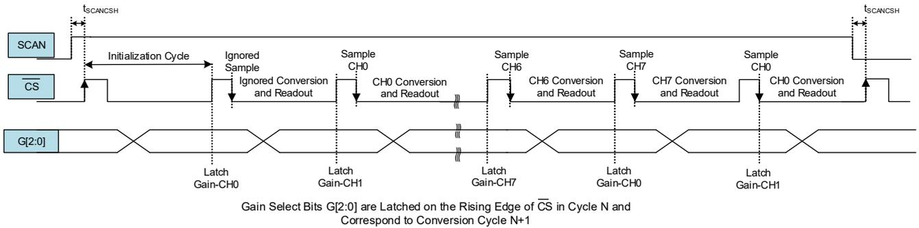
Figure 7. SCAN Timing Diagram - Normal Mode
