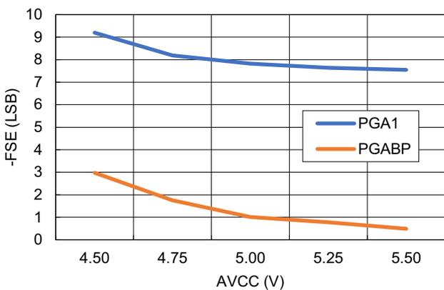
Figure 91. -Full-Scale Error vs AVCC
