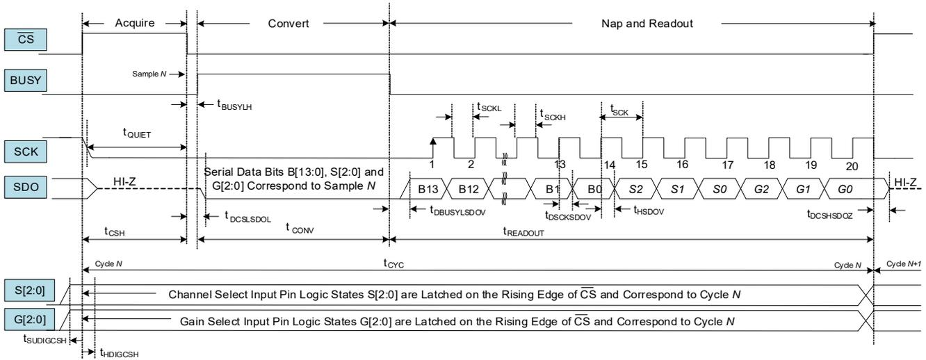
Figure 121. Timing Diagram - Low Power Mode
