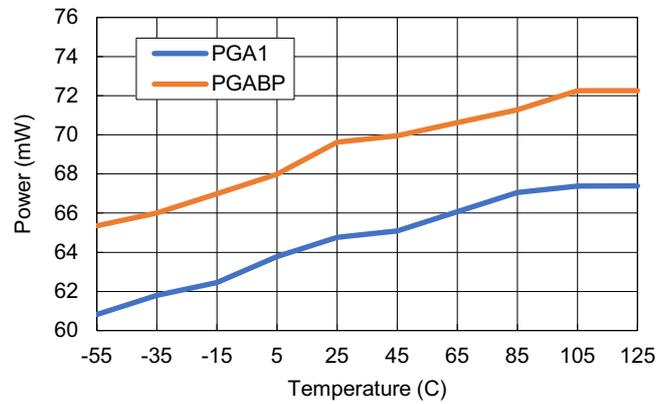
Figure 84. Power vs Temperature
