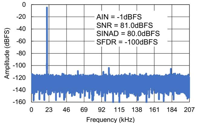
Figure 62. 32k FFT - 20.3kHz, PGA = 1
