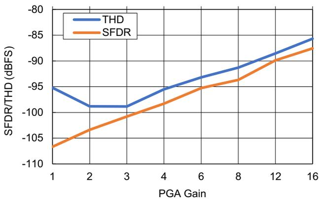
Figure 73. THD and SFDR vs PGA Gain
