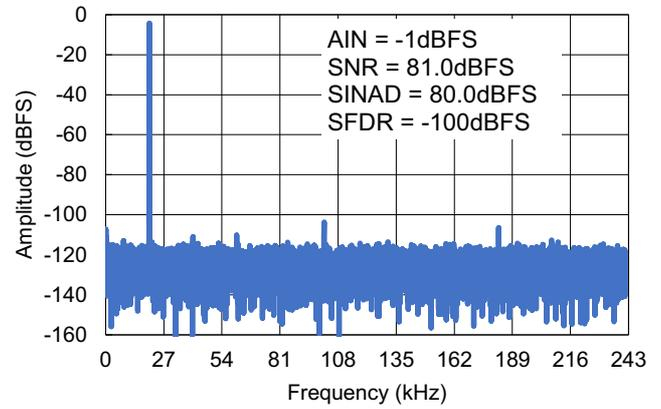
Figure 19. 32k FFT - 20.3kHz, PGA = 1
