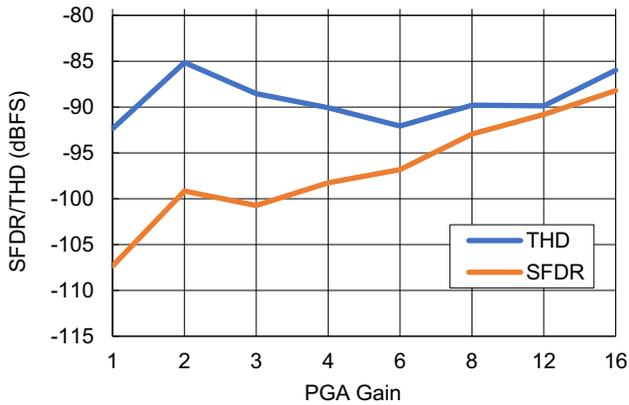
Figure 116. THD and SFDR vs PGA Gain
