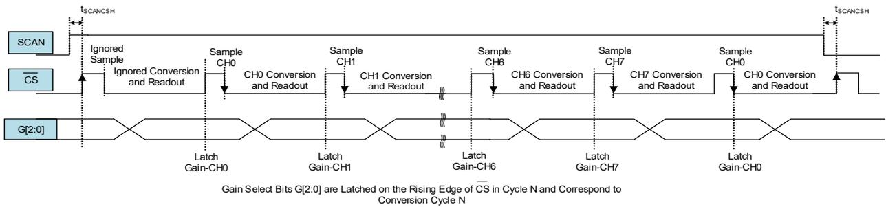
Figure 9. SCAN Timing Diagram - Low Power Mode
