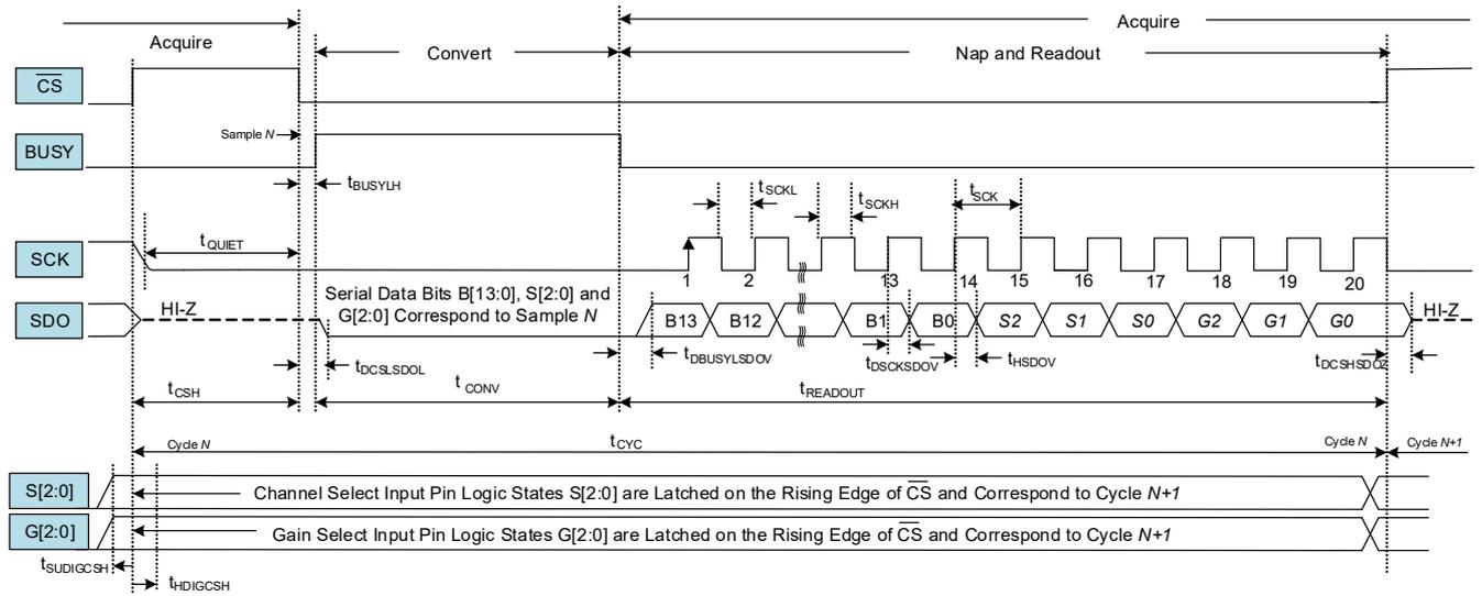
Note: Bits S2, S1, S0, G2, G1, and G0 are optional and not required. For maximum sample rate, do not provide additional clocks for these bits.
