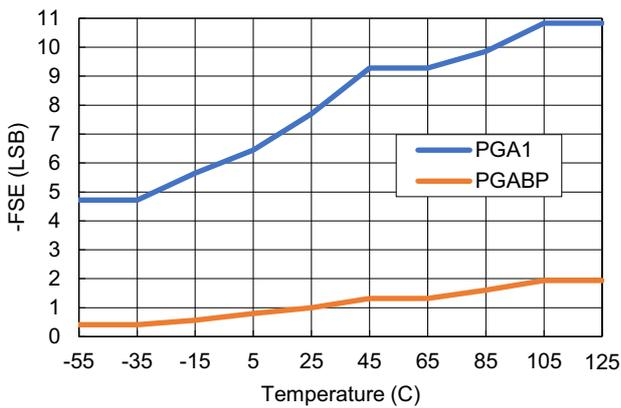
Figure 50. -Full-Scale Error vs Temperature
