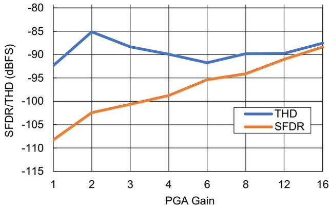
Figure 104. THD and SFDR vs PGA Gain
