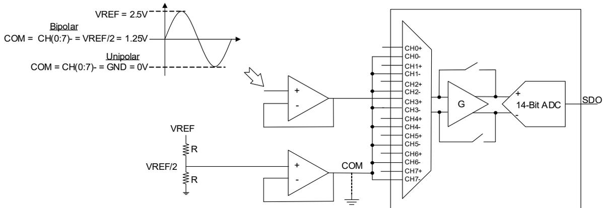
Figure 130. Single-Ended Application Schematic
