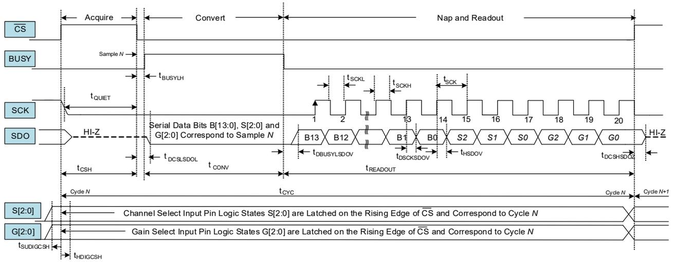
Note: Bits S2, S1, S0, G2, G1, and G0 are optional and not required. For maximum sample rate, do not provide additional clocks for these bits.
