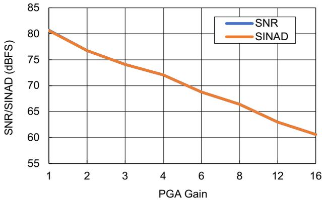
Figure 28. SNR and SINAD vs PGA Gain
