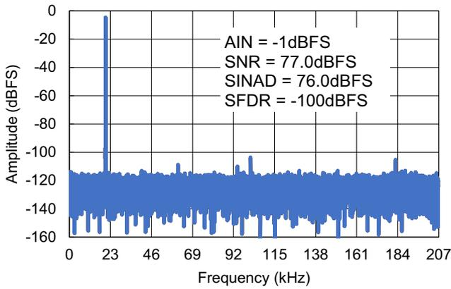
Figure 63. 32k FFT - 20.3kHz, PGA = 2
