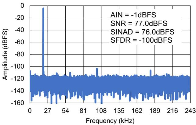
Figure 20. 32k FFT - 20.3kHz, PGA = 2
