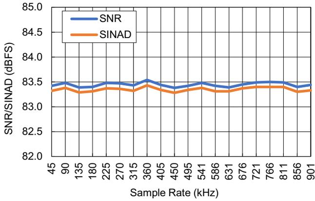
Figure 34. SNR and SINAD vs Sample Rate
