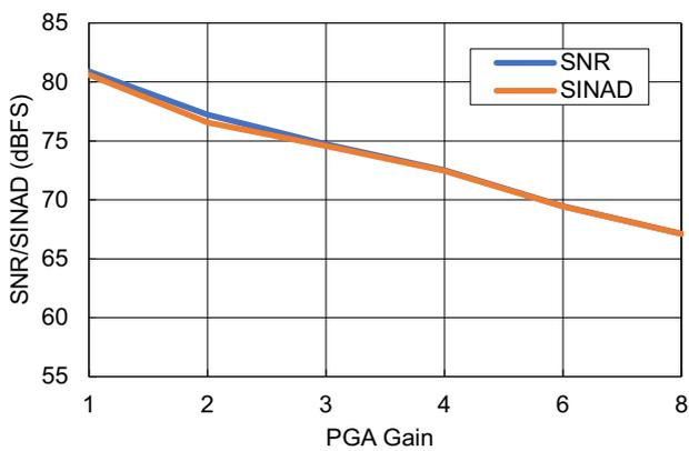
Figure 114. SNR and SINAD vs PGA Gain
