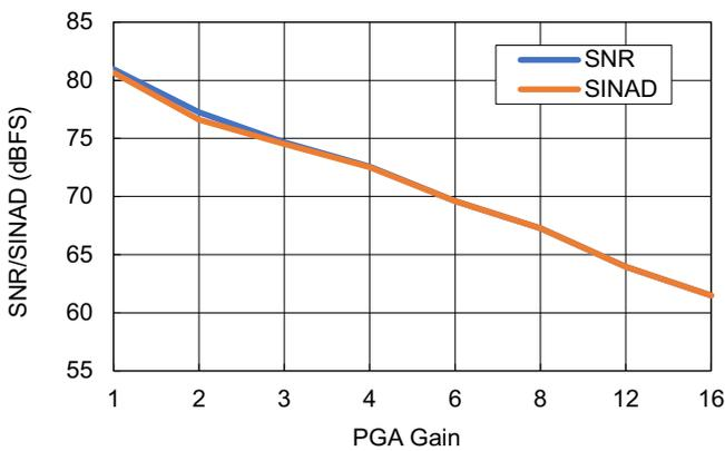
Figure 102. SNR and SINAD vs PGA Gain
