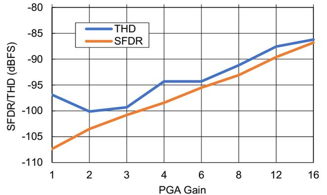
Figure 29. THD and SFDR vs PGA Gain
