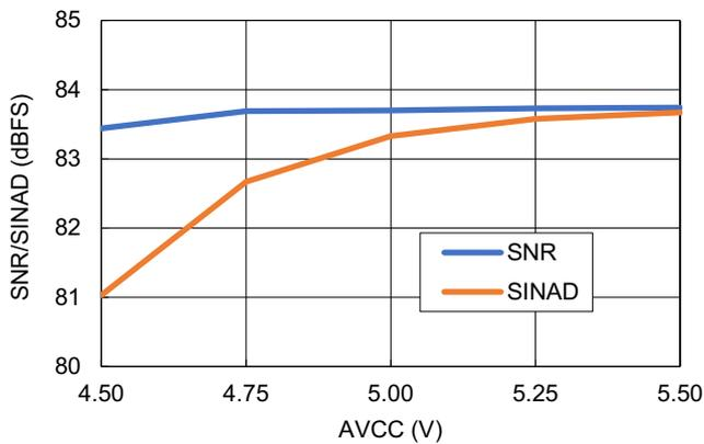
Figure 108. SNR and SINAD vs AVCC
