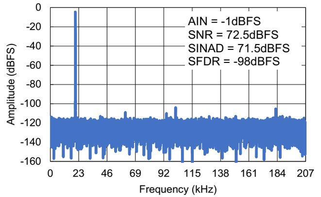
Figure 64. 32k FFT - 20.3kHz, PGA = 4
