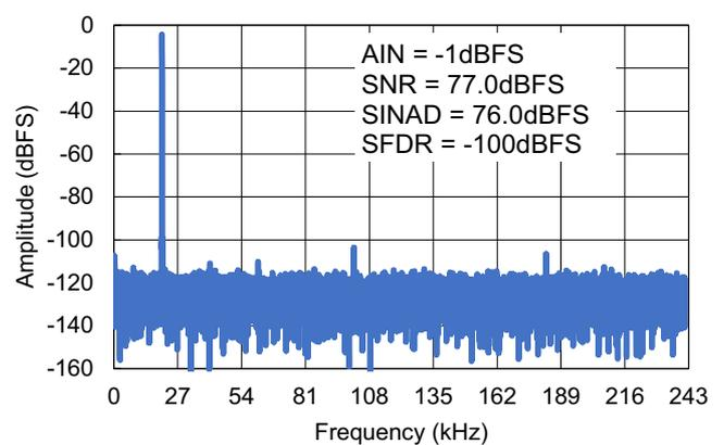
Figure 21. 32k FFT - 20.3kHz, PGA = 4
