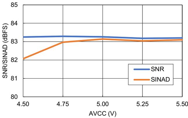
Figure 65. SNR and SINAD vs AVCC
