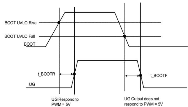
Figure 9. BOOT UVLO to UG Propagation Delay
