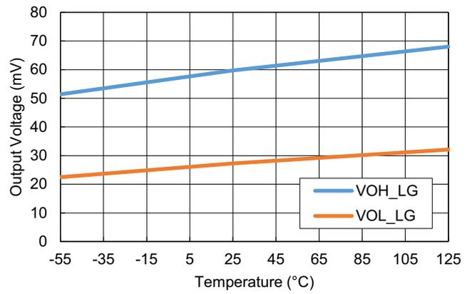
Figure 35. Low-Side Driver V<sub>OL</sub> and V<sub>OH</sub> vs Temperature; 100mA load
