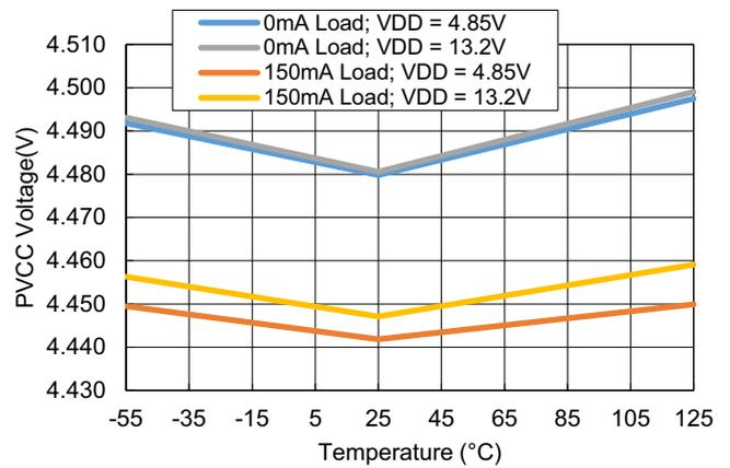
Figure 25. PVCC vs Temperature; PVCC = 4.5V
