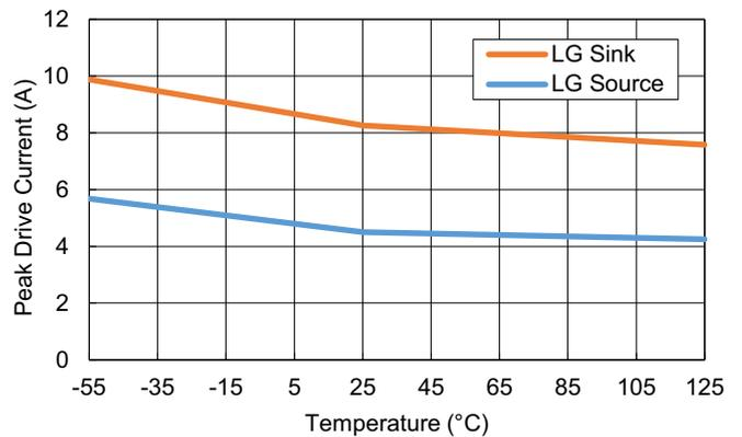
Figure 37. Low-Side Driver Peak Source and Sink Current vs Temperature
