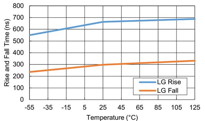
Figure 39. Rise and Fall Times with 470nF on UG and 1000nF on LG vs Temperature; 30% to 70%
