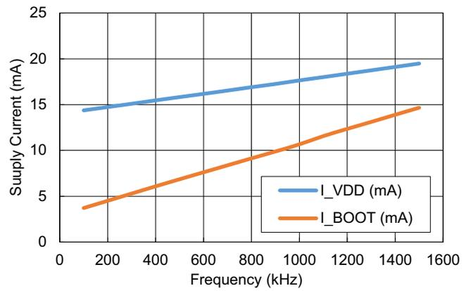
Figure 48. VDD and BOOT Dynamic Operating Current vs f<sub>SW</sub>; VDD = PHS = 12V; PVCC = BOOT-PHS = 4.5V;
