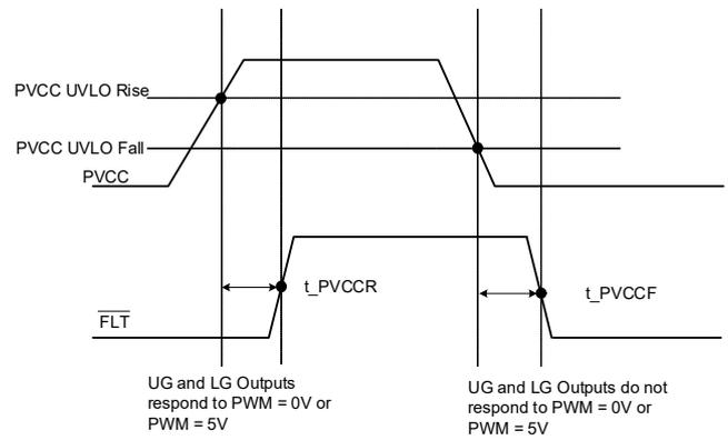
Figure 7. PVCC UVLO to FLT Propagation Delay
