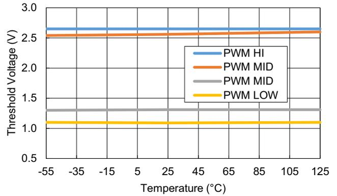
Figure 31. PWM Thresholds vs Temperature
