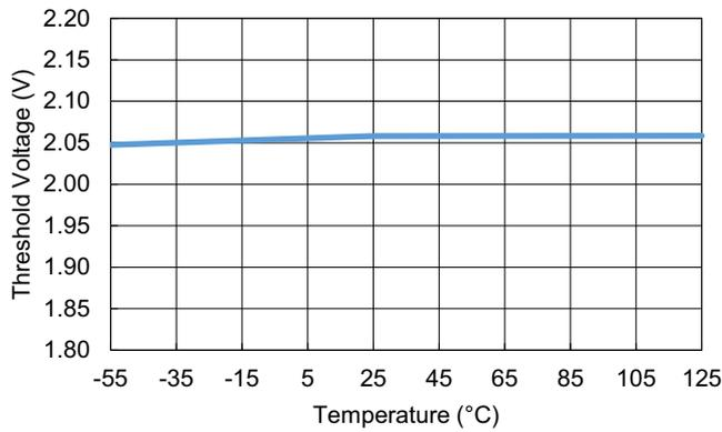
Figure 30. PWM Pin Float Voltage Vs Temperature
