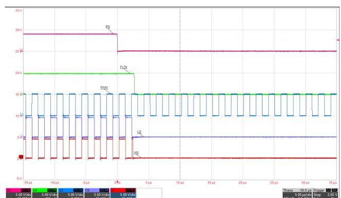
Figure 45. EN Falling Transient Response
