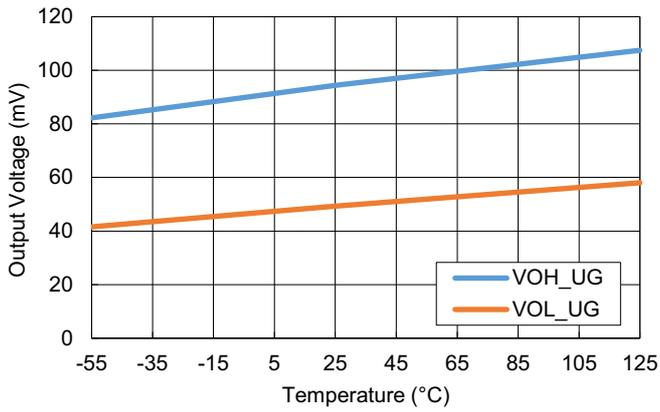
Figure 34. High-Side Driver V<sub>OL</sub> and V<sub>OH</sub> vs Temperature; 100mA load
