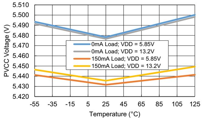
Figure 23. PVCC vs Temperature; PVCC = 5.5V
