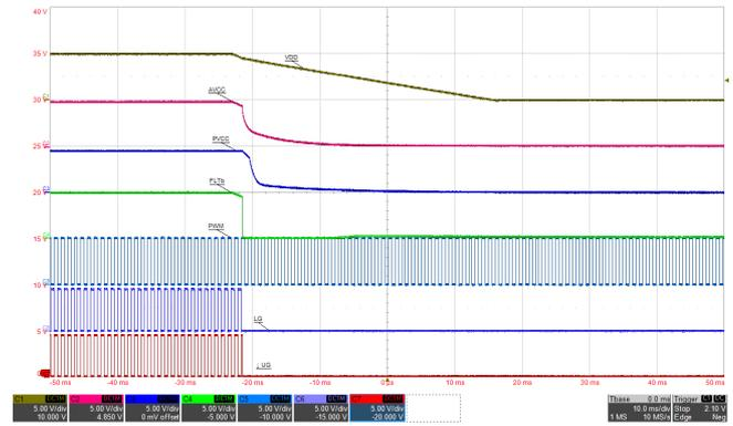
Figure 43. VDD Power-Down Sequence with EN = VDD
