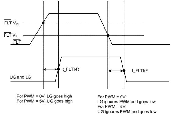
Figure 11. FTLb Propagation Delay (External Driven)
