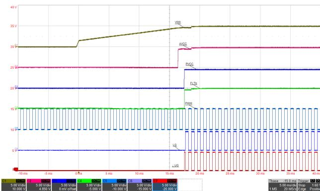
Figure 42. VDD Power-Up Sequence with EN = VDD
