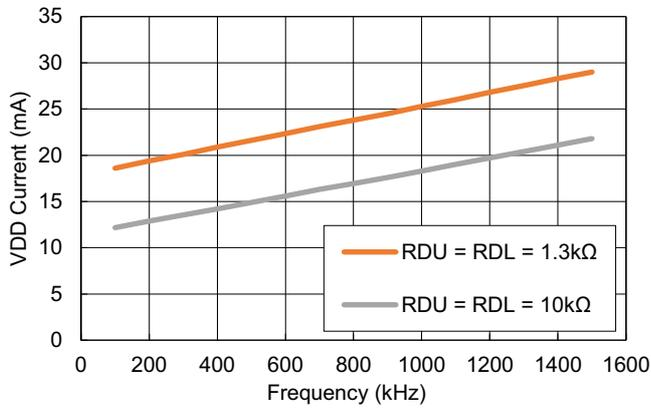
Figure 47. VDD Dynamic Operating Current vs f<sub>SW</sub>;
