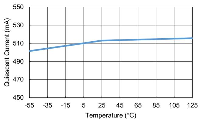
Figure 21. BOOT Static Bias Current vs Temperature;
