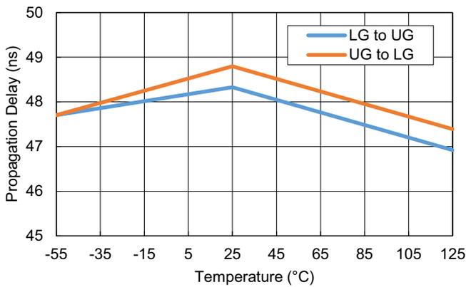
Figure 18. Dead Time Delay vs Temperature;
