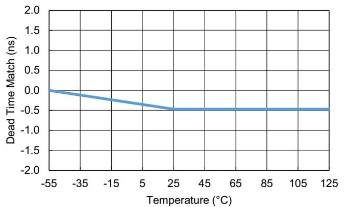
Figure 19. Dead Time Delay Matching vs Temperature;
