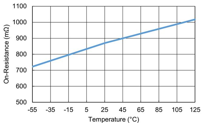
Figure 33. BOOT Switch r<sub>DS(ON)</sub> vs Temperature
