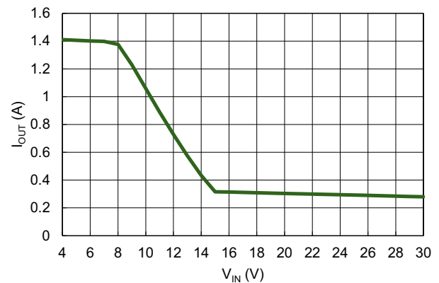
Figure 36. Foldback Current Limit ( I_{OUT} vs V_{IN}-V_{OUT} , V_{OUT} = 0.9V )
