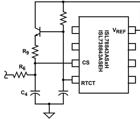
FIGURE 10. SLOPE COMPENSATION
