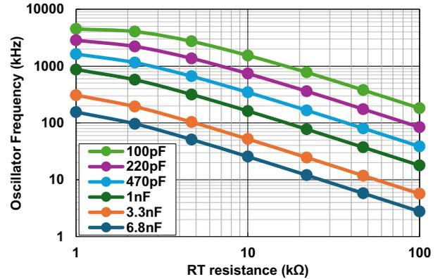
FIGURE 7. OSCILLATOR FREQUENCY vs RT AND CT VALUES
