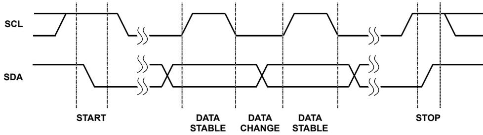
FIGURE 1. VALID DATA CHANGES, START, AND STOP CONDITIONS
