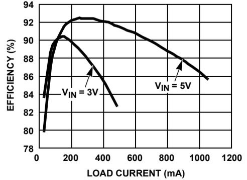
FIGURE 2. BOOST EFFICIENCY AT  $V_{OUT} = 12V$  (P MODE)
