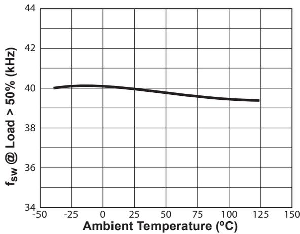
Figure 7.3 : Switching Frequency vs. Temperature<sup>1</sup>
