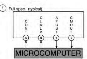
This type usesCONT,CLALV,AFOUT,CMOUTterminal as I/F terminal to the microcomputer.
