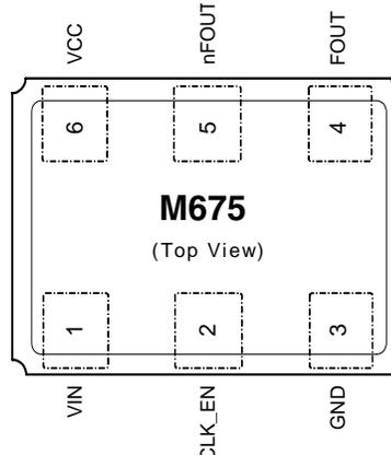
Figure 1: Pin Assignment
