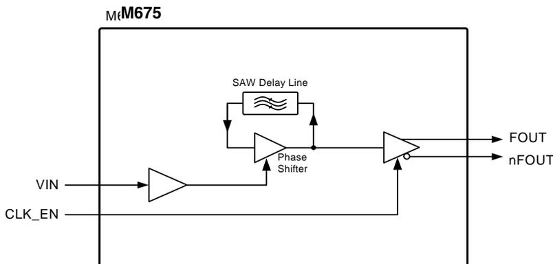
Figure 2: Block Diagram
