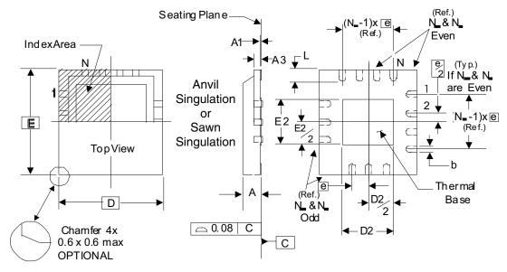
NOTE: The following package mechanical drawing is a generic drawing that applies to any pin count VFQFN package. This drawing is not intended to convey the actual pin count or pin layout of this device. The pin count and pinout are shown on the front page. The package dimensions are in Table 7 below.
