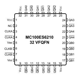
Figure 3. 32-Lead VFQFN Package Pinout (Top View) Figure 3. 32-Lead VFQFN Package Pinout (Top View)
