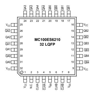
Figure 2. 32-Lead LQFP Package Pinout (Top View)
