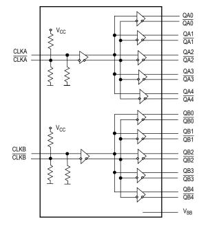
Figure 1. MC100ES6210 Logic Diagram
