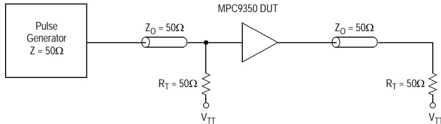
Figure 7. TCLK MPC9350 AC Test Reference for  $V_{CC} = 3.3 \text{ V}$  and  $V_{CC} = 2.5 \text{ V}$
