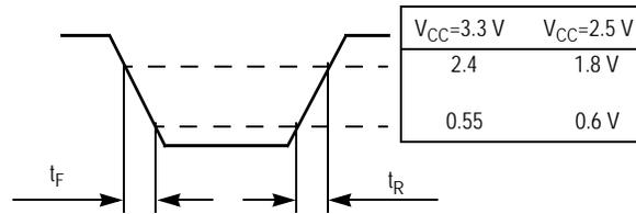
The time from the maximum low level voltage to minimum high level of a clock signal, expressed in ns.
