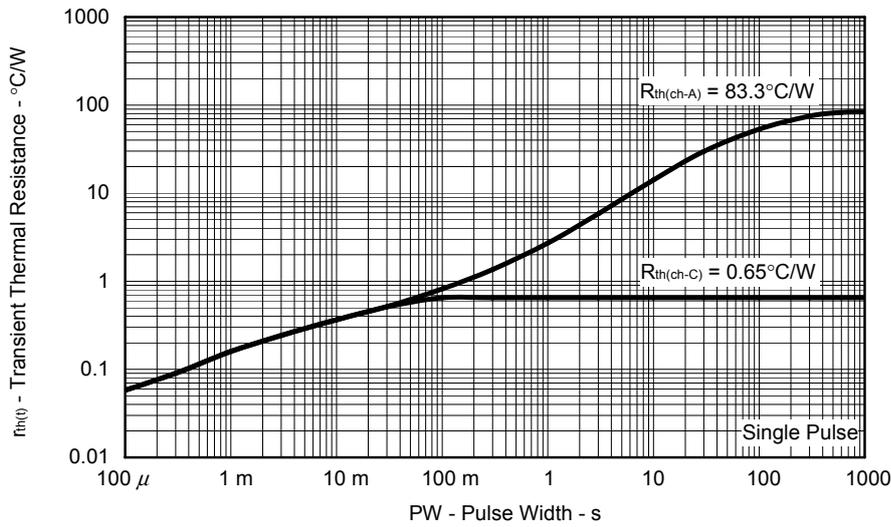
**Note** Confirm the operation tracks are in Safe Operating Area.
