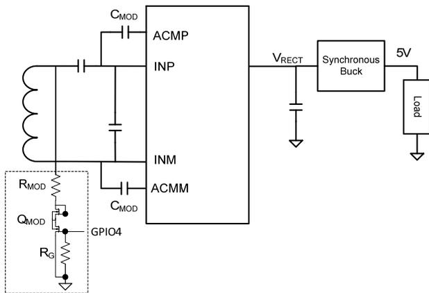
Figure 9: Modulation components
