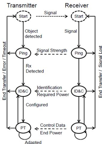
The P9025AC goes through four phases: Start/Selection, Ping, Identification & Configuration, and Power Transfer.
