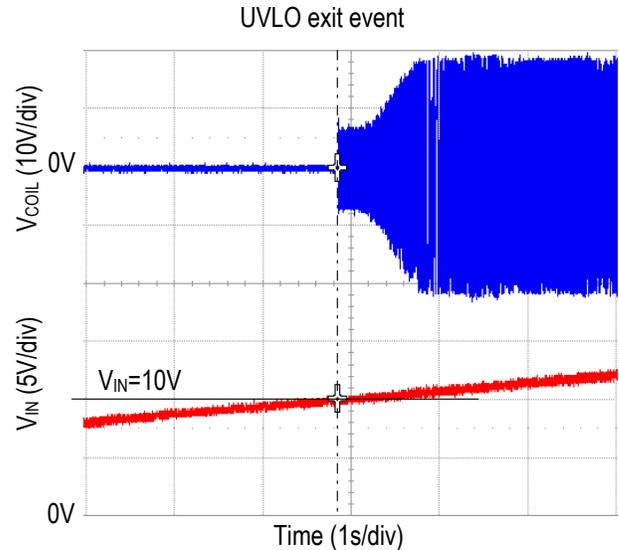
Figure 8. VIN versus UVLO threshold with /EN low.
