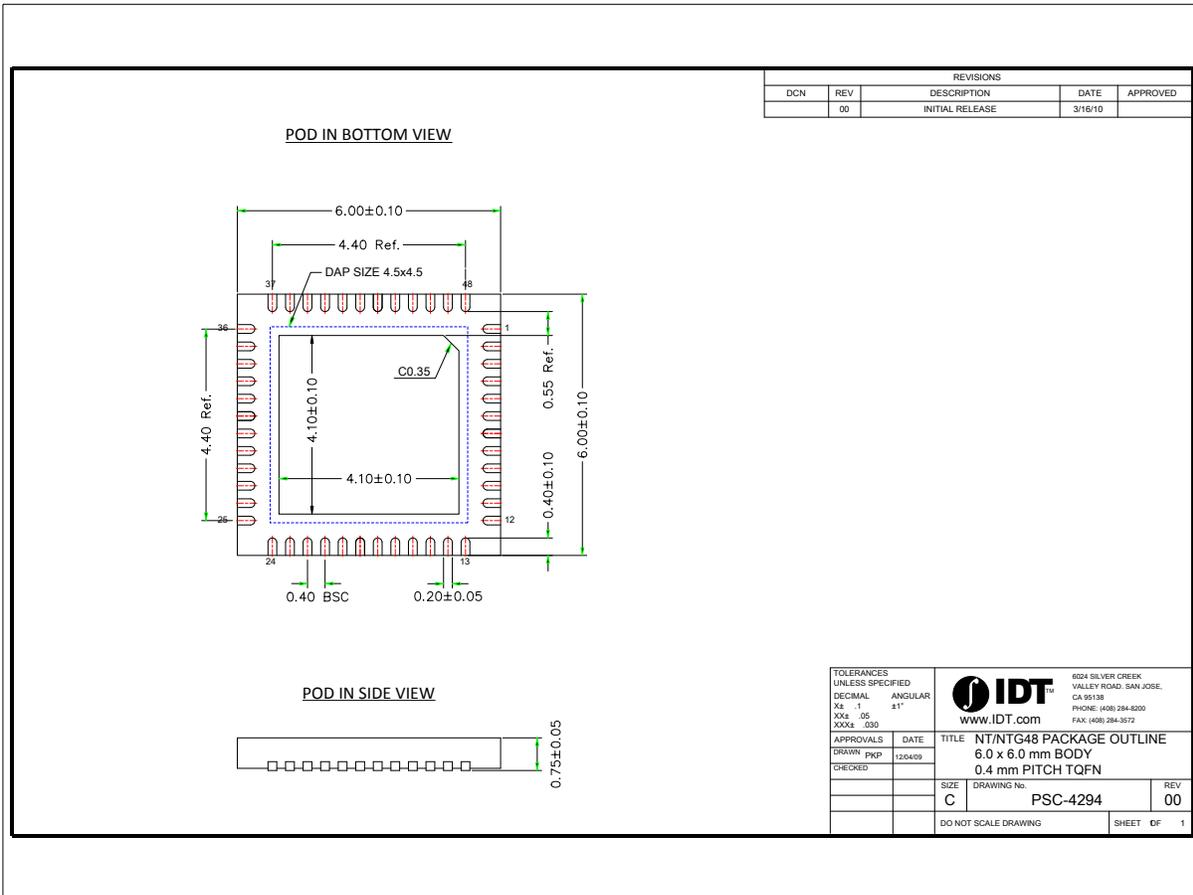
Figure 13. IDTP9036A Package Outline Drawing (NTG48 TQFN-48L 6.0 mm x 6.0 mm x 0.75 mm48L, 0.4mm pitch)
