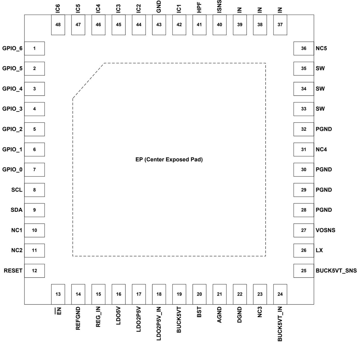
Figure 2. IDTP9036A Pin Configuration (NTG48 TQFN-48L 6.0 mm x 6.0 mm x 0.75 mm, 0.4mm pitch)
