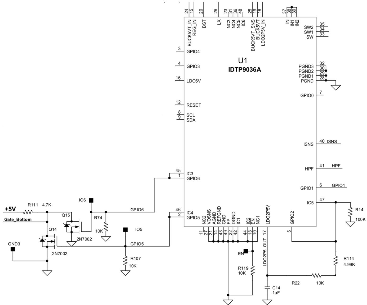
Figure 11b. Wired-NOR using GPIO5 and GPIO6, LDO2P5V
