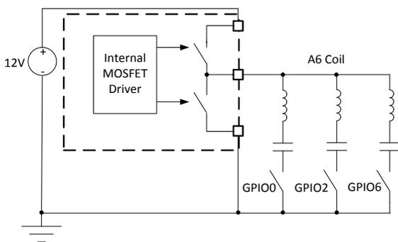
Figure 5 Half Bridge Inverter TX Coil Driver.
