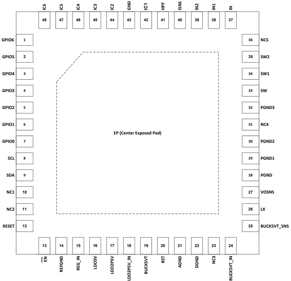
Figure 2 P9036B Pin Configuration (NTG48 TQFN-48L 6.0 mm x 6.0 mm x 0.75 mm, 0.4mm pitch)
