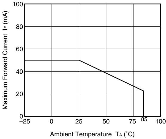
**MAXIMUM LOAD CURRENT vs. AMBIENT TEMPERATURE**
