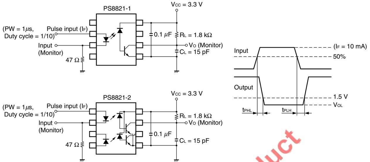
**Remark**  $C_L$  is approximately  $15\text{ pF}$  which includes probe and stray wiring capacitance.
