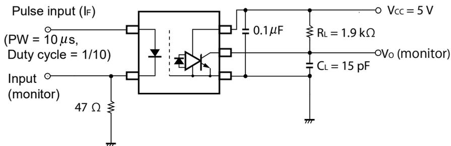
**Remark**  $C_L$  includes probe and stray wiring capacitance.
