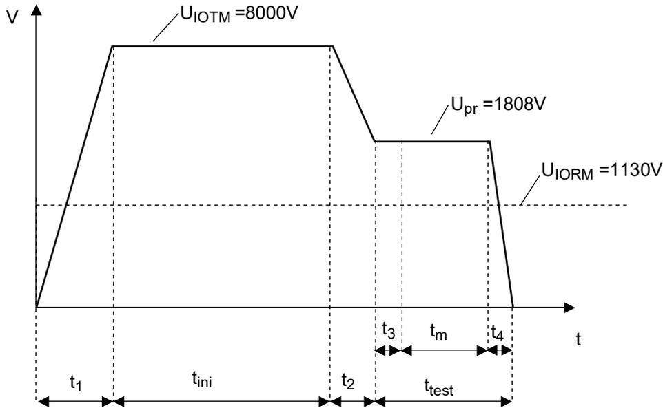
$t_1, t_2 = 1 \text{ to } 10 \text{ sec}$
