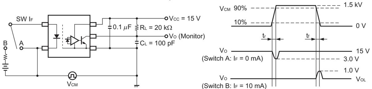
C<sub>L</sub> includes probe and stray wiring capacitance.
