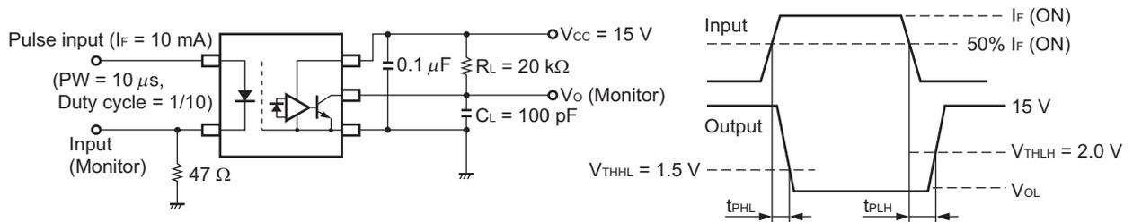
C<sub>L</sub> includes probe and stray wiring capacitance.
