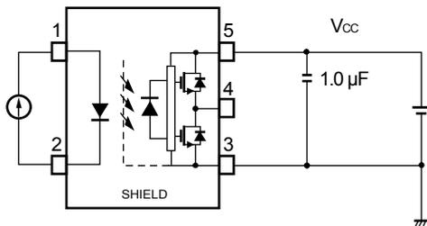
Fig. 6 UVLO Test Circuit
