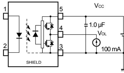
Fig. 5  $I_{CCH}/I_{CCL}$  Test Circuit
