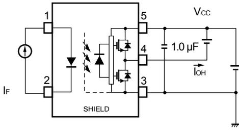
Fig. 2  $I_{OL}$  Test Circuit
