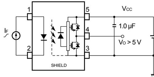
**Fig. 8 t<sub>PLH</sub>, t<sub>PHL</sub>, t<sub>r</sub>, t<sub>f</sub> Test Circuit and Wave Forms**
