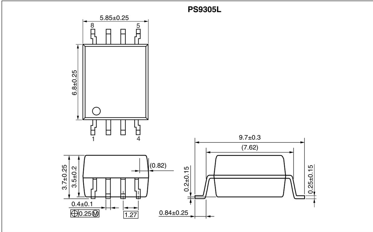
Lead Bending Type (Gull-wing) for Long Clearance Distance (Surface Mount)
