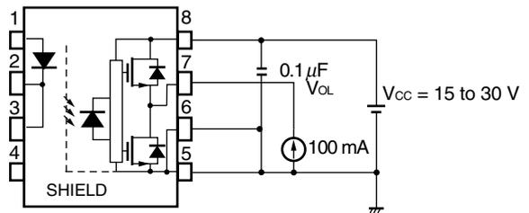
Fig. 5  $I_{FLH}$  Test Circuit
