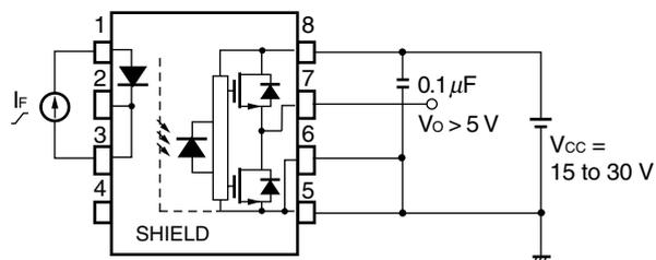
Fig. 6 UVLO Test Circuit
