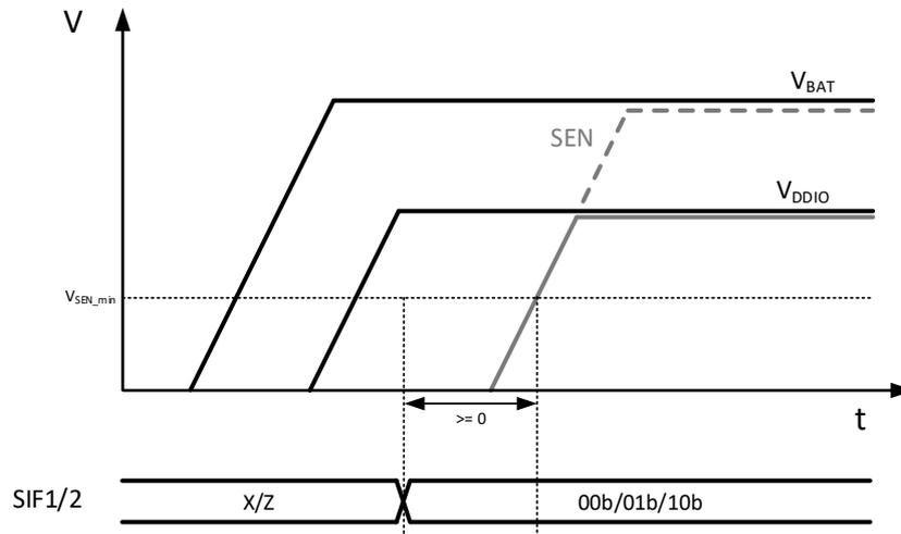
**Figure 4: Supply Ramping Up (SEN at logic-low)**
