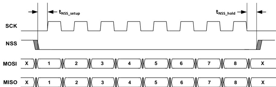
Figure 8: SPI mode 0 (CPOL, CPHA = 0)
