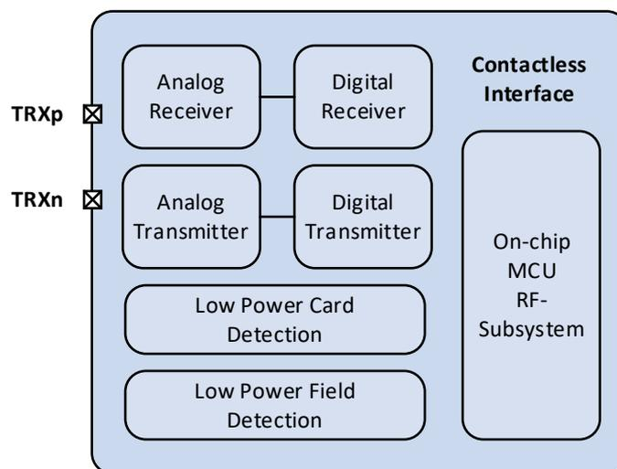
Figure 6: Contactless Interface
