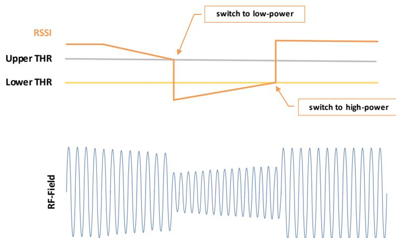
Figure 7: Dynamic Digital Power Control (DDPC)
