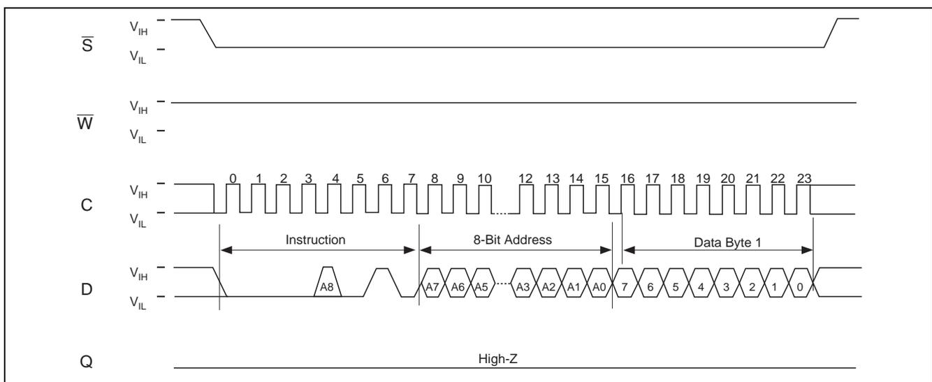
Note: 1. Depending on the memory size, as shown in Address Range Bits table, the most significant address bit is don't care.
