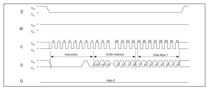
Note: 1. Depending on the memory size, as shown in Address Range Bits table, the most significant address bits are don't care.
