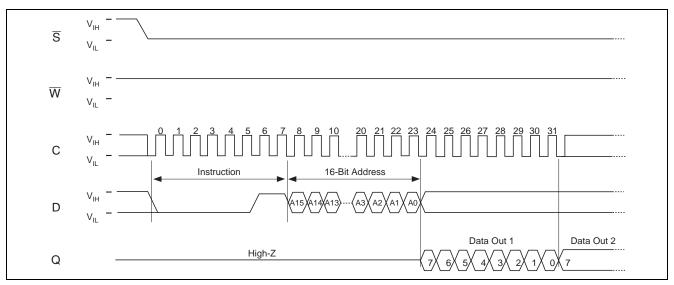
Note: 1. Depending on the memory size, as shown in the following table, the most significant address bits are don't care
