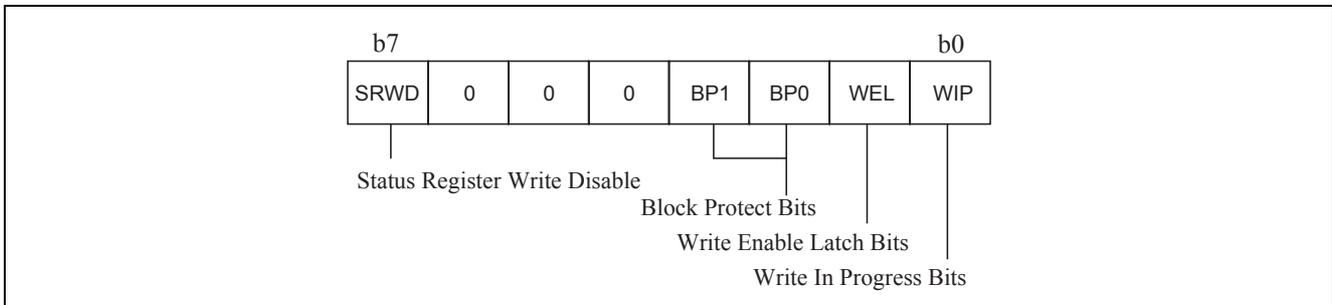
**WIP bit:** The Write In Progress (WIP) bit indicates whether the memory is busy with a Write or Write Status Register cycle.
