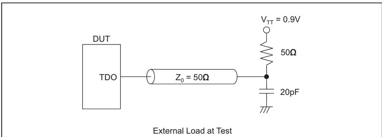
**TAP AC Operating Characteristics**(T<sub>A</sub> = -40 to +85°C, V<sub>DD</sub> = 1.8V ±0.1V)
