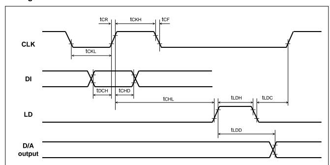
(Note) Timing chart above is a schematic representation of the timing of each signal type. CLK signal input is High or Low regardless, LD signal High input is enabled.
