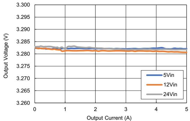
Figure 6. Load Regulation, 3.3V V<sub>OUT</sub>, 400kHz, HTSSOP
