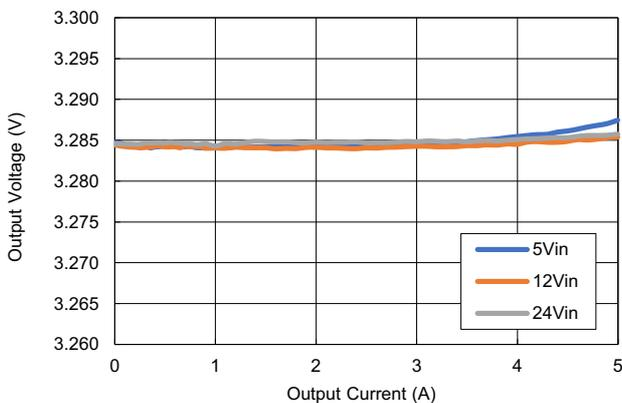
Figure 5. Load Regulation, 3.3V V<sub>OUT</sub>, 400kHz, QFN
