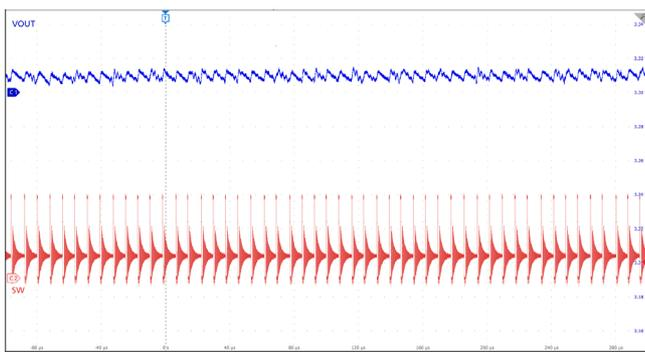
Figure 11. Steady State, 3.3V V<sub>OUT</sub>, No Load, 400kHz, QFN
