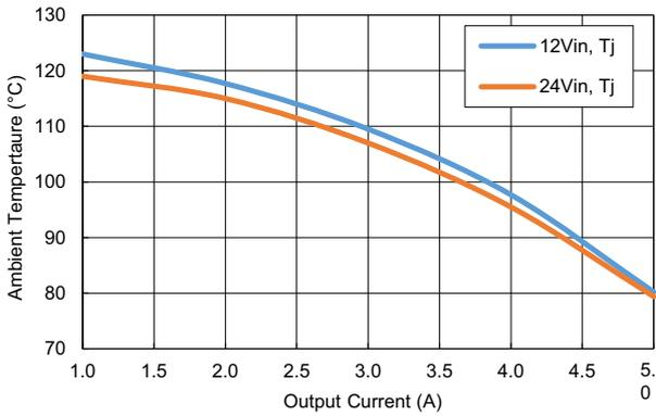
Figure 19. Safe Operating Area: 3.3V<sub>out</sub>, 400kHz, HTSSOP, Default EVM
