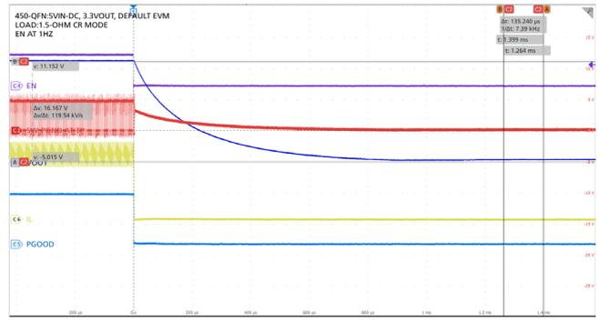
Figure 8. EN Shutdown, 5V<sub>IN</sub>, 3.3V V<sub>OUT</sub>, 400kHz, 1.5Ω Load, QFN
