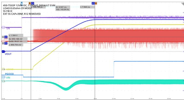
Figure 9. External SS, 12V<sub>IN</sub>, 3.3V<sub>OUT</sub>, 0.65Ω Load, C<sub>SS</sub> = 39nF, HTSSOP
