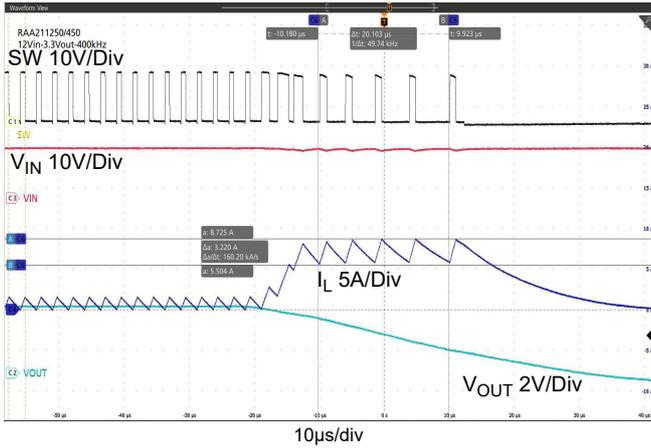
Figure 25. Short Output Protection, High-Side OC Protection
