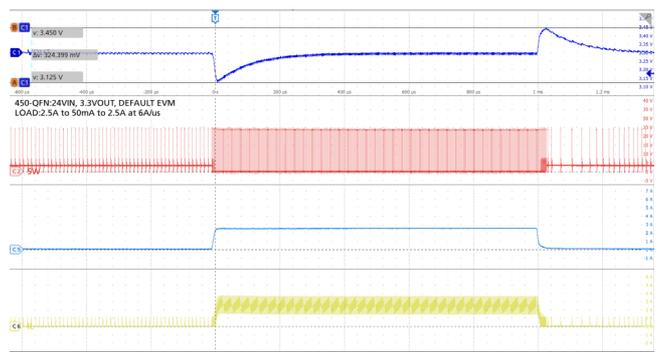
Figure 12. Load Transient, 24V<sub>IN</sub>, 3.3V<sub>OUT</sub>, 400kHz, 50mA to 2.5A, QFN
