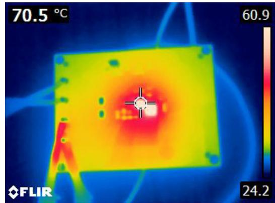
Figure 20. Thermal Image, 12V<sub>IN</sub>, 3.3V<sub>OUT</sub>, 400kHz, 5A, QFN, T<sub>J</sub> = 70.5°C
