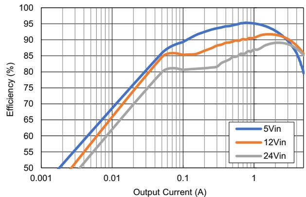
Figure 4. Efficiency vs Load, 3.3V V<sub>OUT</sub>, 400kHz, HTSSOP
