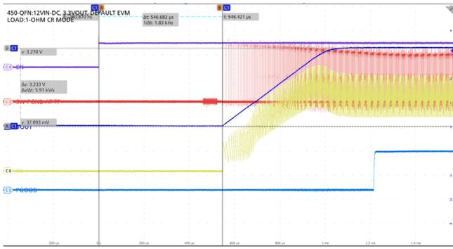
Figure 7. EN Start-Up, 12V<sub>IN</sub>, 3.3V V<sub>OUT</sub>, 400kHz, 1.0Ω Load, QFN
