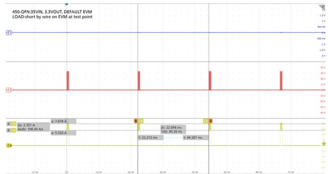
Figure 16. Output Short Protection with Hiccup, QFN
