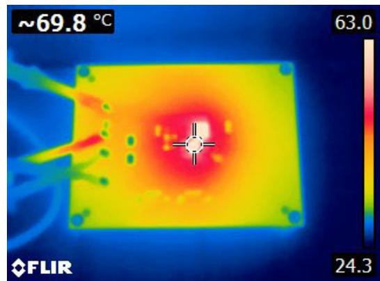
Figure 22. Thermal Image, 12V<sub>IN</sub>, 3.3V<sub>OUT</sub>, 400kHz, 5A, HTSSOP, T<sub>J</sub> = 69.8°C
