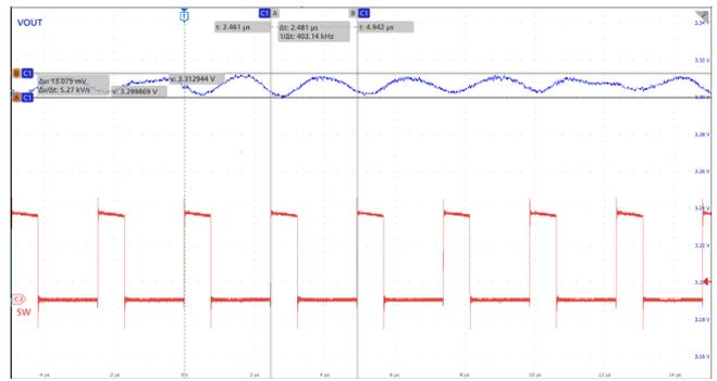
Figure 10. Steady State, 3.3V V<sub>OUT</sub>, Full Load, 400kHz, QFN
