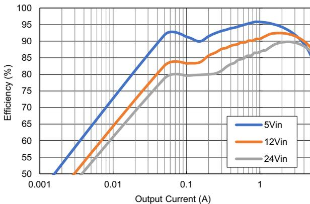
Figure 3. Efficiency vs Load, 3.3V V<sub>OUT</sub>, 400kHz, QFN
