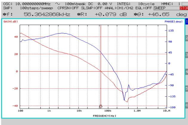
Figure 17. 24V<sub>IN</sub>, 2A, F<sub>c</sub> = 56kHz, PM = 47° at -40°C
