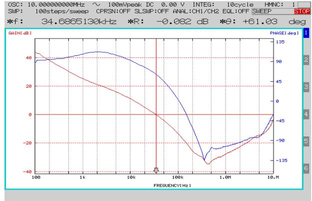
Figure 16. 24V<sub>IN</sub>, 2A, F<sub>c</sub> = 35kHz, PM = 61° at 85°C
