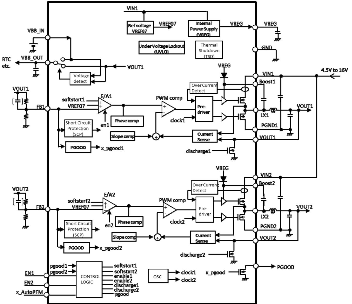
RAA23023x (2CH DCDC, VOUT set by external resistors)
