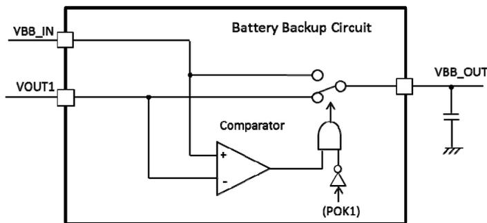
Note : POK1 is an IC internal signal which identifies CH1 operating status. It cannot be seen from IC outside.
