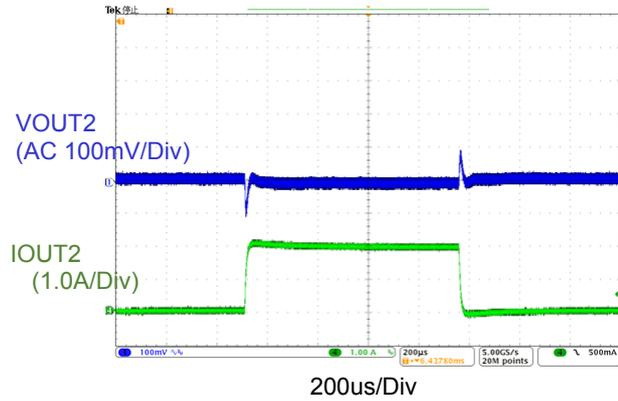
**Battery Backup circuit : VBB\_OUT changing Waveform (RAA23022x)**
