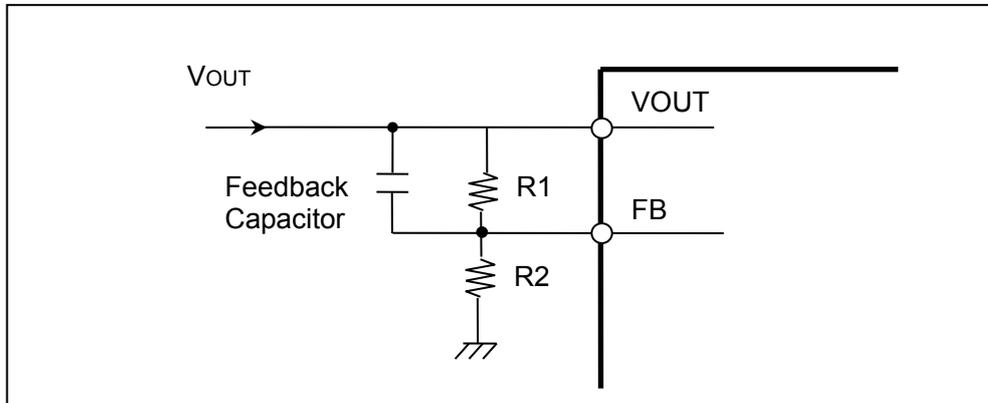
When using feedback capacitor with an output voltage fixed product, connect feedback capacitor between VOUT pin and FB pin.
