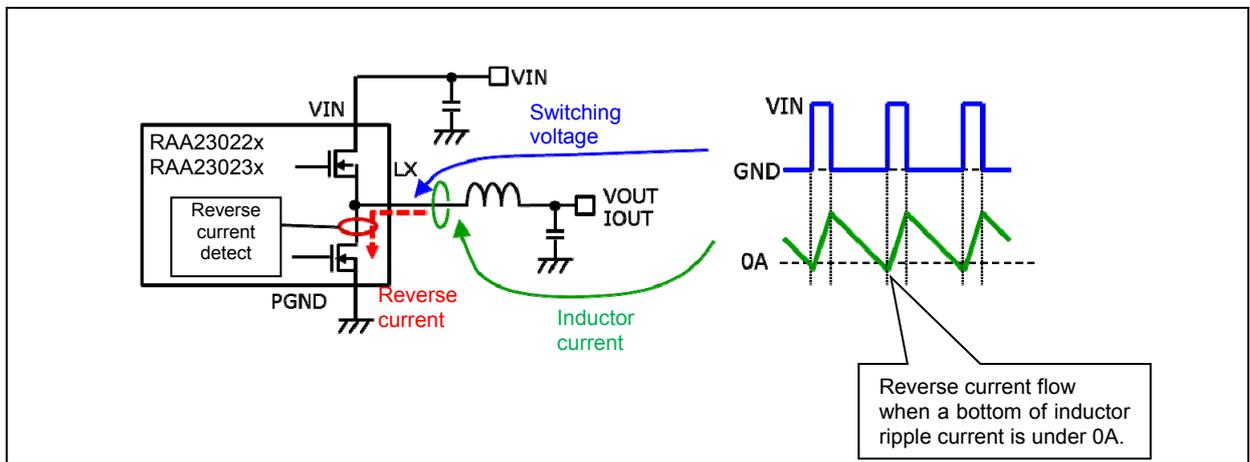
RAA23022x and RAA23023x have x\_autoPFM pin. When Low level, the devices operate Auto PFM mode (PFM mode / PWM mode changed automatically). When High level, the devices operate PWM mode, then not change into Auto PFM mode.
