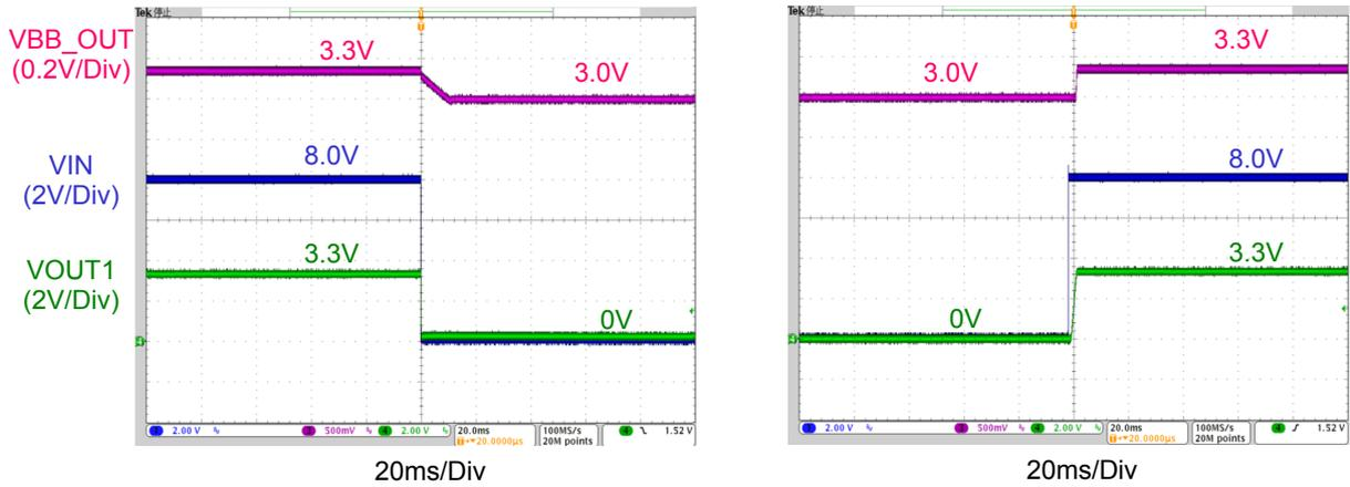
(2) Battery Voltage(VBB\_IN pin) = 3.6V、 VOUT1=3.3V
