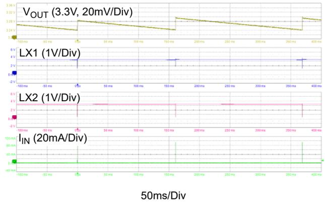
Figure 19. Steady State, PFM mode, Load = 3.3MΩ
