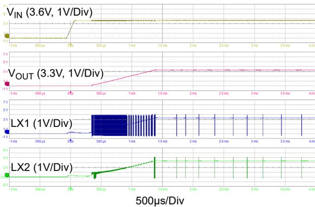
Figure 16. Soft-Start with Fast VIN Ramp Rate
