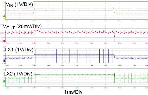
Figure 20. Line Transient:  $V_{OUT} = 3.3V$ ; 1mA Load
