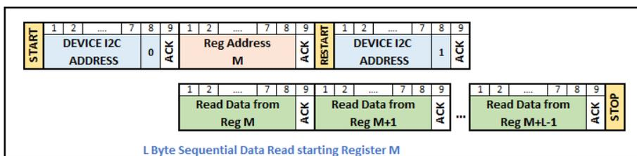
Figure 35. Sequential Data Read Starting at Register M
