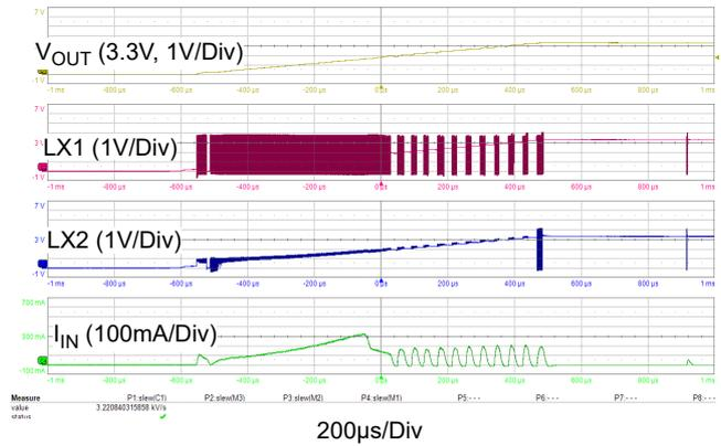
Figure 15. Inrush Current:  $V_{IN} = 3.6V$ ,  $V_{OUT} = 3.3V$
