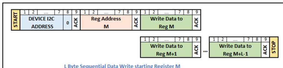
Figure 33. Sequential Data Write Starting at Register M
