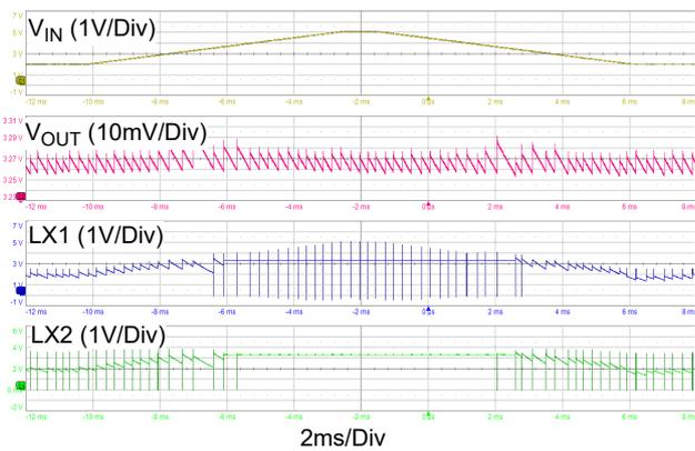
Figure 24. Buck-Boost Transition:  $V_{OUT} = 3.3V$ ; Load = 1mA, PFM mode
