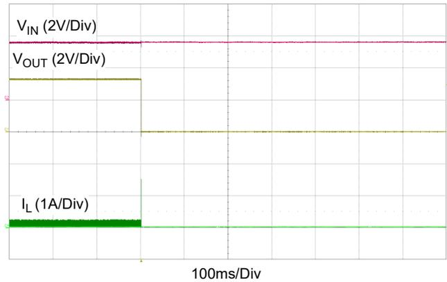
Figure 27. Output Short-Circuit Behavior; Shutdown Mode
