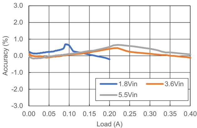
Figure 10. Output Voltage Accuracy vs. Load Current,  $V_{OUT} = 3.3V$
