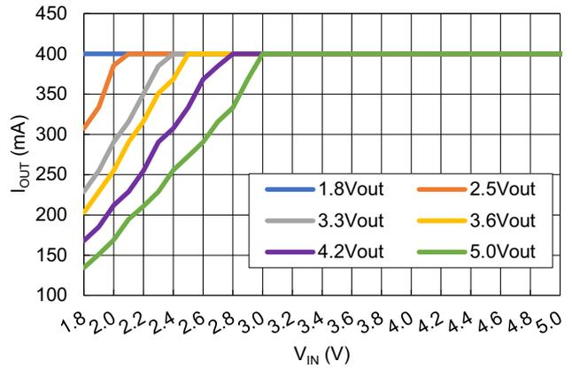
Figure 9. Maximum Load Current vs. Input Voltage
