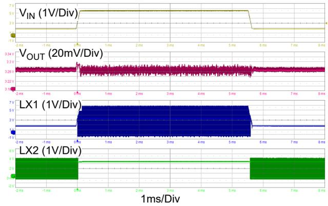
Figure 21. Line Transient:  $V_{OUT} = 3.3V$ ; 130mA Load
