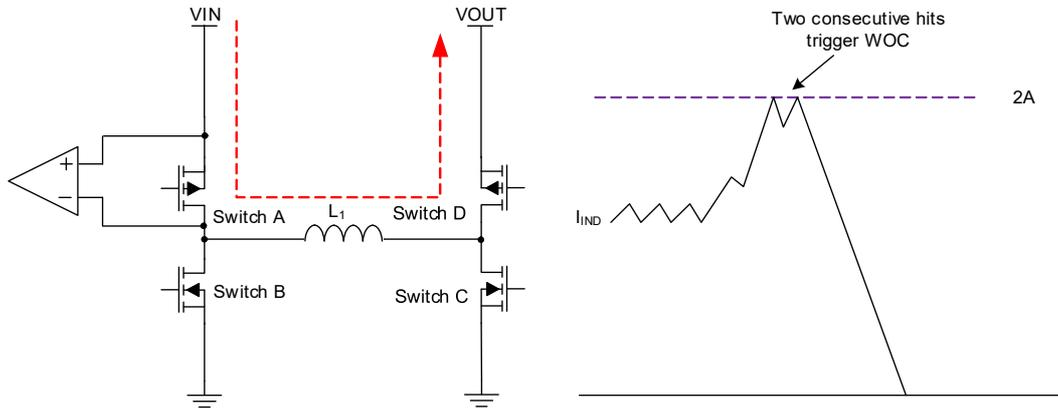
Figure 30. Overcurrent Protection
