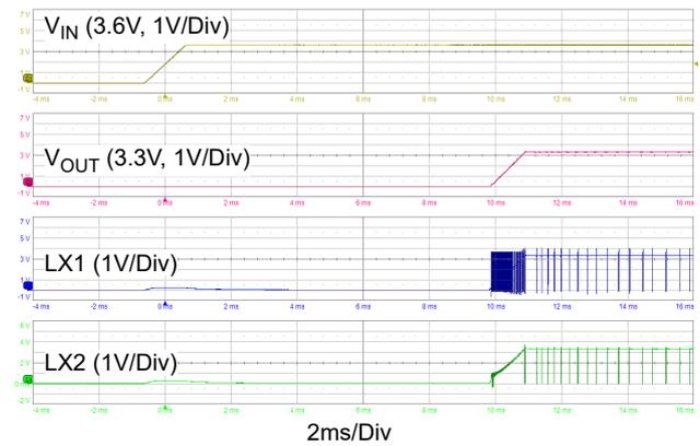
Figure 17. Soft-Start with Slow VIN Ramp Rate
