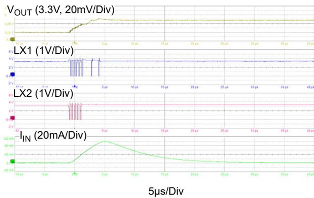
Figure 18. Steady State, PFM mode, Load = 3.3MΩ
