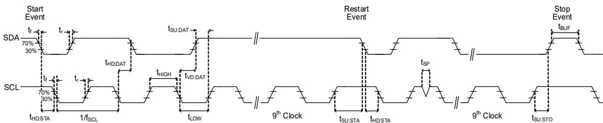
Figure 36. I<sup>2</sup>C Timing
