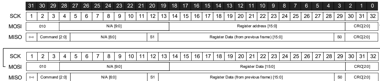
Figure 21. SafeSPI Frame for Writing Register Data
