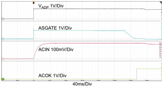
Figure 7. Adapter Insertion,  $V_{ADP}$ : 0V → 5V,  $V_{BAT}$  = 18V, ChargeCurrent = 0.256A
