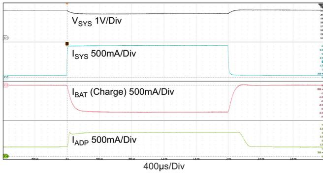
**Figure 23. Boost Mode: Output Voltage Loop ↔ Adapter Current Loop,  $V_{ADP} = 5V$ ,  $MaxSystemVoltage = 21V$ ,  $V_{BAT} = 20.5V$ ,  $AdapterCurrentLimit = 3A$ ,  $ChargeCurrent = 0A$ ,  $SystemLoad: 0.2A \leftrightarrow 4A$**
