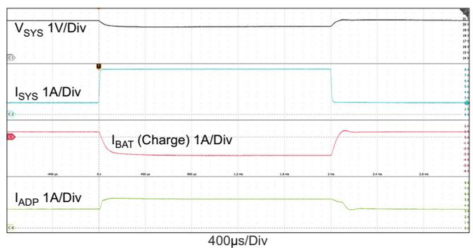
**Figure 26. Buck-Boost Mode: Charge Current Loop ↔ Adapter Current Loop,  $V_{ADP} = 20V$ ,  $MaxSystemVoltage = 21V$ ,  $V_{BAT} = 20V$ ,  $AdapterCurrentLimit = 5A$ ,  $ChargeCurrent = 1A$ ,  $SystemLoad: 2A \leftrightarrow 8A$ ,  $Buck\_Boost\_CCM\_stretch\_period = 2x$**
