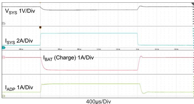
**Figure 27. Buck Mode: Output Voltage Loop ↔ Adapter Current Loop,  $V_{ADP} = 28V$ ,  $MaxSystemVoltage = 21V$ ,  $V_{BAT} = 20.5V$ ,  $AdapterCurrentLimit = 5A$ ,  $ChargeCurrent = 0A$ ,  $SystemLoad: 2A \leftrightarrow 12A$**
