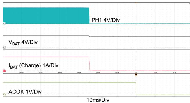
Figure 9. Adapter Removal,  $V_{ADP}$ : 28V → 0V,  $V_{BAT}$  = 18V, ChargeCurrent = 6A
