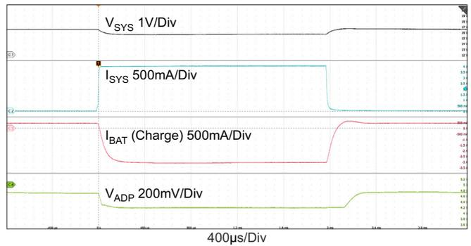
**Figure 30. Boost Mode: Charge Current Loop ↔ Input Voltage Loop,  $V_{ADP} = 5V$ ,  $MaxSysVoltage = 21V$ ,  $V_{BAT} = 16V$ ,  $InputVoltageLimit = 4.096V$ ,  $ChargeCurrent = 0.5A$ ,  $SystemLoad: 0A \leftrightarrow 4A$**
