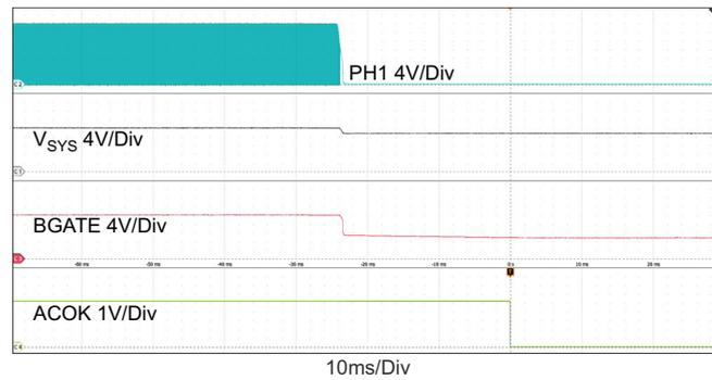
Figure 20. Adapter Removal,  $V_{ADP}$ : 28V → 0V,  $V_{BAT}$  = 18V, SystemLoad = 2A
