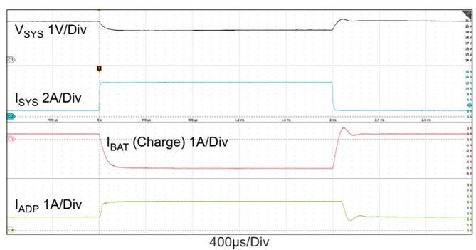
**Figure 28. Buck Mode: Charge Current Loop ↔ Adapter Current Loop,  $V_{ADP} = 28V$ ,  $MaxSystemVoltage = 21V$ ,  $V_{BAT} = 20V$ ,  $AdapterCurrentLimit = 5A$ ,  $ChargeCurrent = 1A$ ,  $SystemLoad: 2A \leftrightarrow 12A$**
