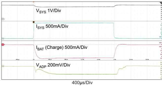
**Figure 29. Boost Mode: Output Voltage Loop ↔ Input Voltage Loop,  $V_{ADP} = 5V$ ,  $MaxSystemVoltage = 21V$ ,  $V_{BAT} = 20.5V$ ,  $InputVoltageLimit = 4.096V$ ,  $ChargeCurrent = 0A$ ,  $SystemLoad: 0A \leftrightarrow 4A$**
