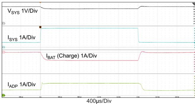
**Figure 25. Buck-Boost Mode: Output Voltage Loop ↔ Adapter Current Loop,  $V_{ADP} = 20V$ ,  $MaxSystemVoltage = 21V$ ,  $V_{BAT} = 20.5V$ ,  $AdapterCurrentLimit = 5A$ ,  $ChargeCurrent = 0A$ ,  $SystemLoad: 2A \leftrightarrow 8A$ ,  $Buck\_Boost\_CCM\_stretch\_period = 2x$**
