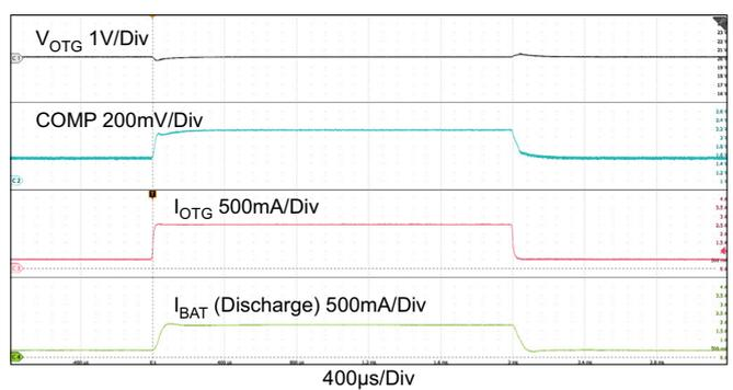
**Figure 17. OTG Mode Transients,  $V_{BAT} = 29.4V$ ,  $V_{OTG} = 20V$ , OTG Load: 0.5A ↔ 3A**
