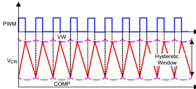
Figure 43. R3 Modulator Operation Principles In Steady State
