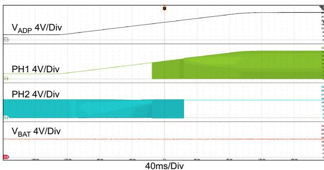
Figure 10. Adapter Voltage Ramp Up, Boost → Buck-Boost → Buck Operation Mode Transitions
