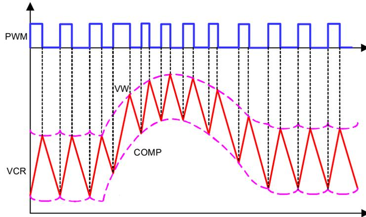
Figure 44. R3 Modulator Operation Principles In Dynamic Response
