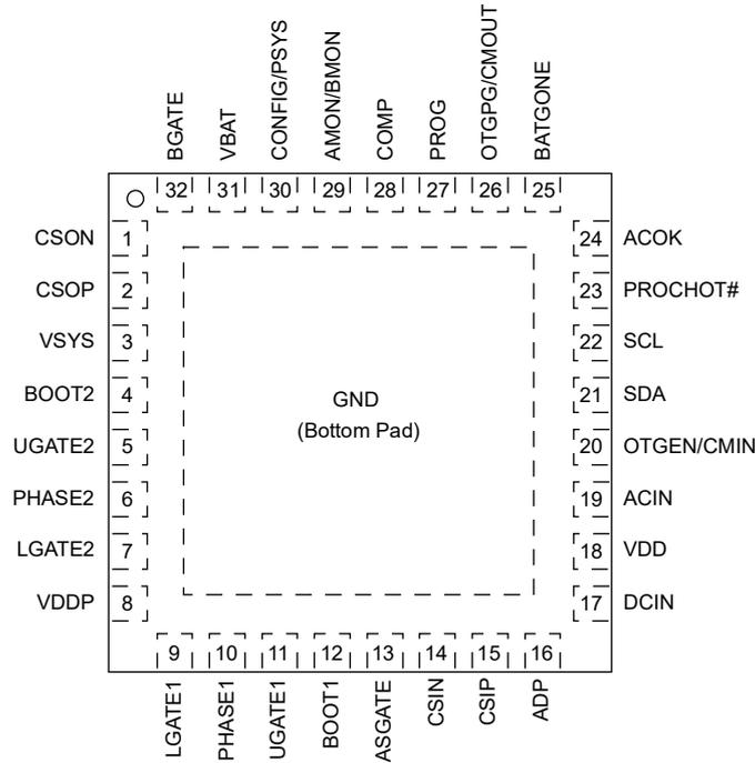
Figure 5. Pin Assignments – Top View
