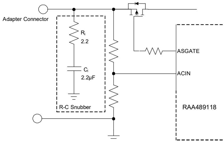
Figure 49. Adapter Input R-C Snubber Circuit
