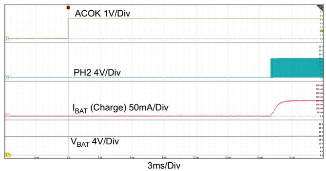
Figure 8. Adapter Insertion,  $V_{ADP}$ : 0V → 5V,  $V_{BAT}$  = 18V, ChargeCurrent = 0.256A (Figure 7 Zoomed In)
