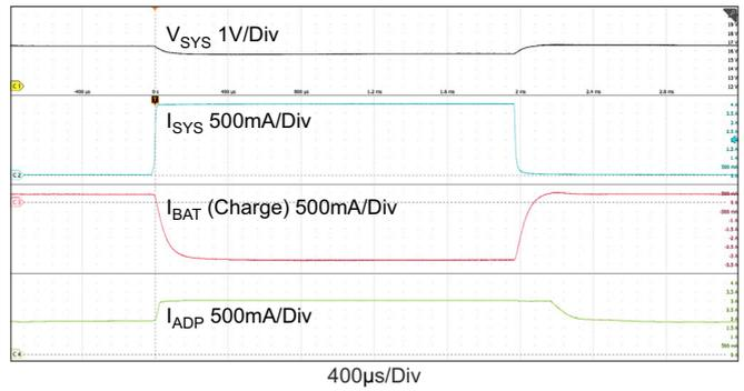
**Figure 24. Boost Mode: Charge Current Loop ↔ Adapter Current Loop,  $V_{ADP} = 5V$ ,  $MaxSystemVoltage = 21V$ ,  $V_{BAT} = 16V$ ,  $AdapterCurrentLimit = 3A$ ,  $ChargeCurrent = 0.5A$ ,  $SystemLoad: 0A \leftrightarrow 4A$**
