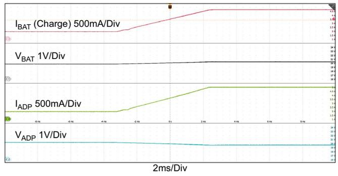
**Figure 13. Buck\_Boost Mode: Charge Current Loop to Adapter Current Loop,  $V_{ADP} = 20V$ ,  $V_{BAT} = 19V$ , AdapterCurrentLimit = 5A, ChargeCurrent: 2A → 6A Buck\_Boost\_CCM\_stretch\_period = 2x**
