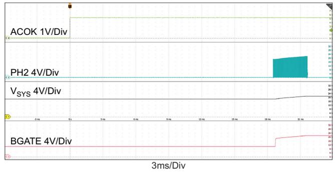
Figure 19. Adapter Insertion,  $V_{ADP}$ : 0V → 5V,  $V_{BAT}$  = 18V, ChargeCurrent = 0A
