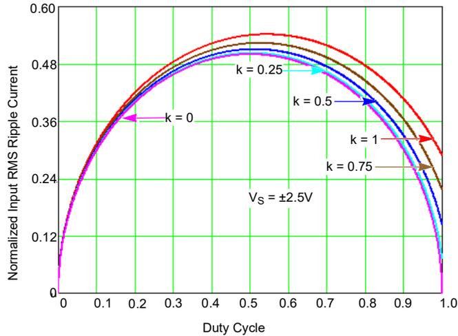
Figure 48. Normalized RMS Input Current at EFF = 1
