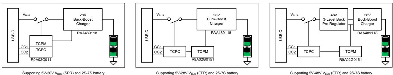
Figure 1. Full-Featured Architecture Solutions Enabled by RAA489118
