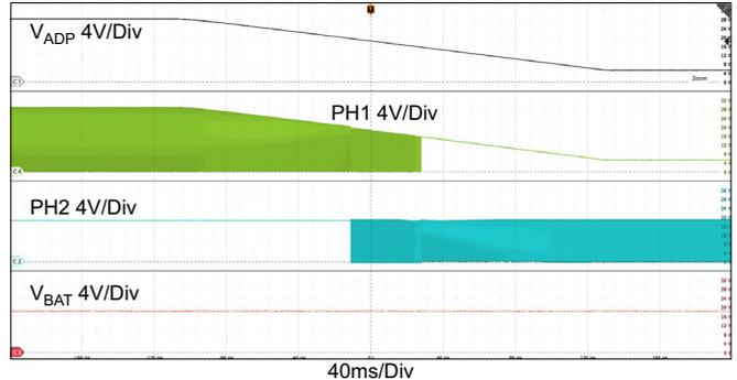
Figure 11. Adapter Voltage Ramp Down, Buck → Buck-Boost → Boost Operation Mode Transitions
