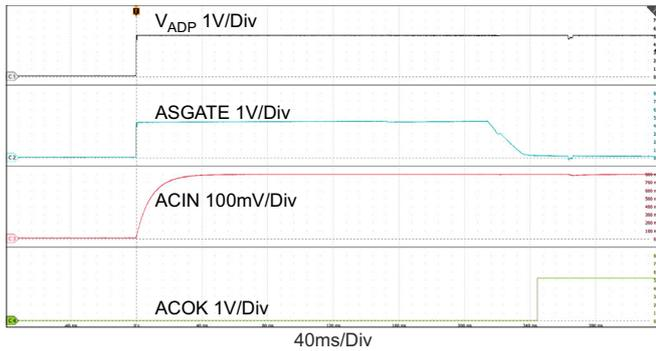
Figure 18. Adapter Insertion,  $V_{ADP}$ : 0V → 5V,  $V_{BAT}$  = 18V, ChargeCurrent = 0A
