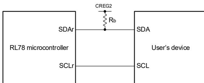
Simplified I<sup>2</sup>C mode connection diagram (during communication at same potential)
