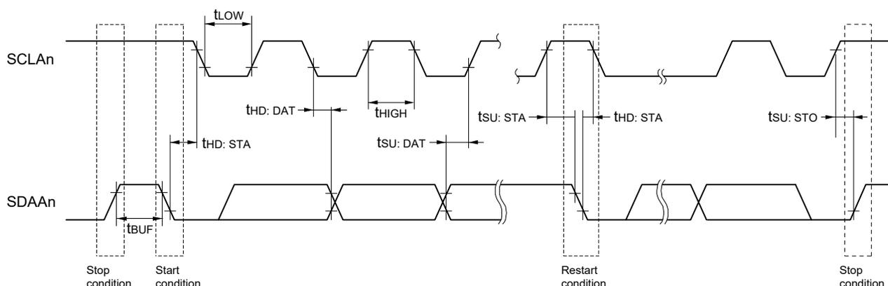
I<sup>2</sup>C serial transfer timing
