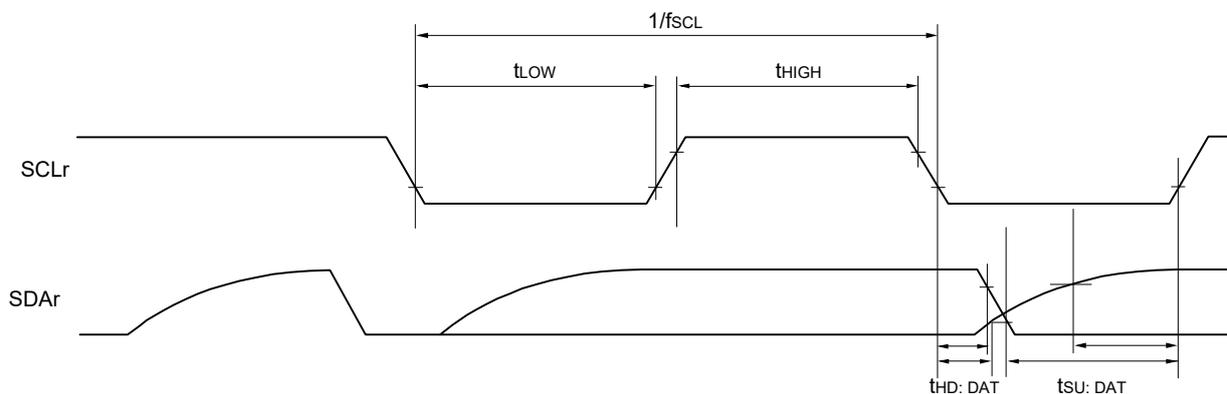
Simplified I<sup>2</sup>C mode serial transfer timing (during communication at same potential)
