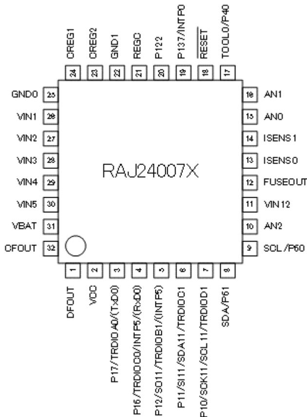
**Caution 1.** REGC pin connects to GND1 pin through a capacitor (0.47 to 1 uF)
